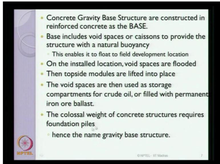
The slide contains a list of bullet points describing the construction and use of concrete gravity base structures. The text is as follows:
