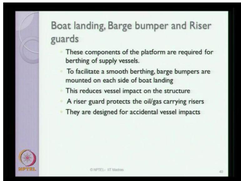
If you look at the boat landing, barge bumpers and riser guards; these are also ancillary components of the platform, which are required for berthing of the supply vessels. To facilitate a smooth berthing, barge bumpers are installed on each side of the boat landing. This reduces the vessel impact on the jacket structure; the riser guard also protects the oil
