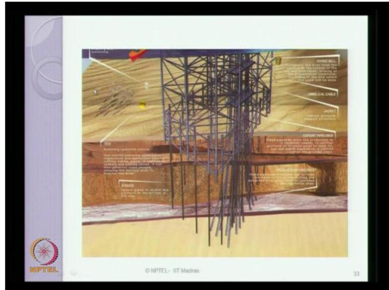
If you look at the subside details of this; these are all the jacket legs what we see here, is also has a remote operated vehicle to see the positioning of the platform. It has got umbilical cables, which are supporting, which are used for the drilling risers, the jacket is what we see here. As the legs and the jackets also has supports derive from the export pipelines and the production pipelines or the product wells, which has been used for exploring oil or producing oil from the seabed.
