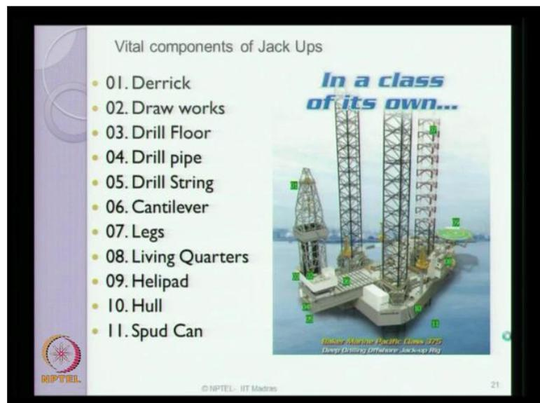
There are vital components of the jack ups, which we must understand for our better knowledge on this kind of marine structure. There are different components marked as one two and so on. I will explain them quickly in the slide here; one is what we call as
