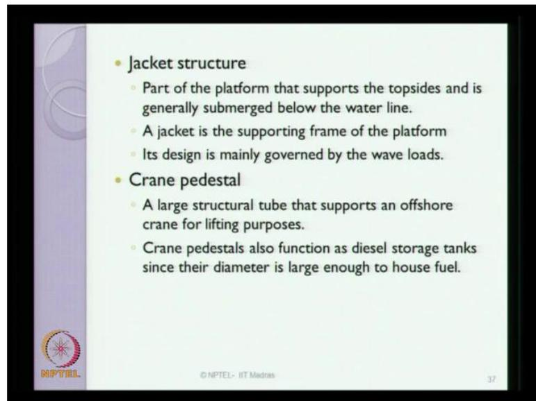
The jacket structure essentially consists of part of the platform, which supports the topside and generally it is submerged below the water. A jacket is a supporting frame of the platform, which is mainly designed to resist the wave loads acting on the platform. Crane pedestal is a large structural tube that supports the offshore crane for lifting purposes. Crane pedestals function also as diesel storage tanks. Since the diameter is large enough to house fuel.
