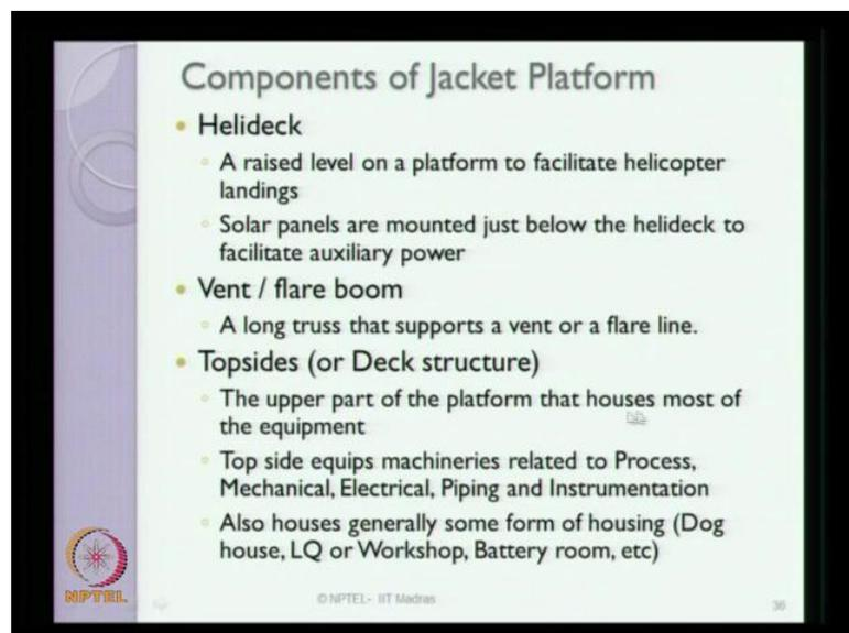
If you look at the components of the jacket platform one by one, helideck is a raised level platform, which facilitates the helipad landing. It houses solar panels, which are mounted just below the helideck to create auxiliary power for production as well as for survival. It contains vent and flare booms is nothing but, a long truss that supports vent
