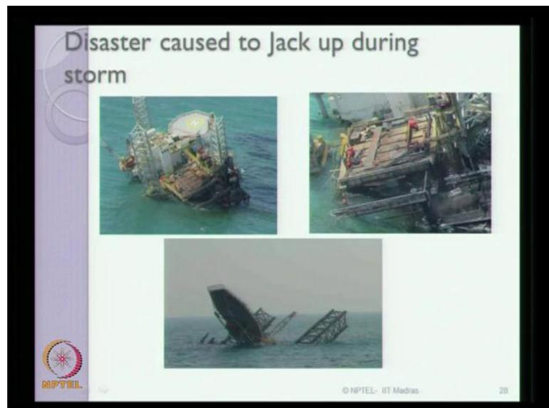
Of course, there are also not avoided from accidents, these are some of the photographs, which show when the disaster caused a jack up rig during a storm condition. These are the three legs, the helipad, the living quarters, and the derricks on the flat or the cranes, which have been actually seen. Can see this complete sink has been an accident caused on a jack up rig during a storm, which we address as a disaster.
