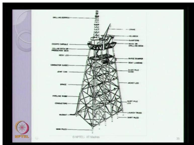
Diagram illustrating the components of a jacket structure:
