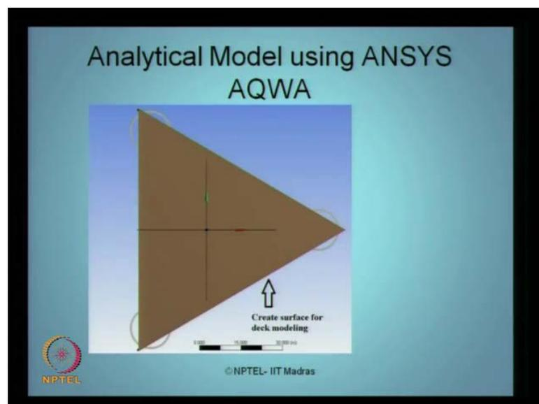
Once the line elements are created then you create the deck using the surface modeling as a deck machine.
