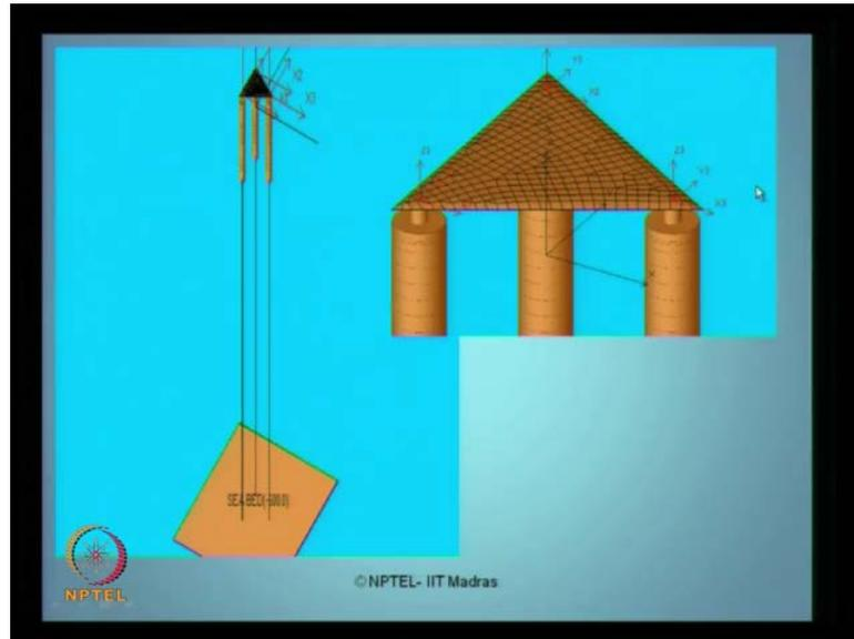
Once this is done then the developed model will be anchored to the sea bed looks like, these are the principle directions of  $X_1$ ,  $X_2$  and  $X_3$ . This may close look of the model, you can see here the ball joint being connected with that of the BLS and the deck here. So, the each one of them have independent coordinate system  $X_1$ ,  $X_2$ ,  $X_3$  and so on so they are independent, one can measure them separately.
