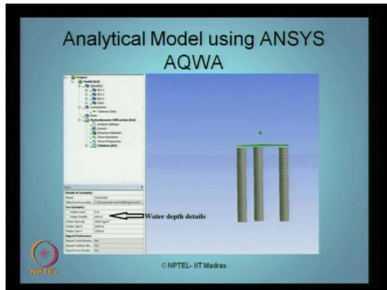
After creating this then the water depth details are given now, this model has been analyzed, to start with at the depth of 600 meter. Of course, this has been tested at the depth of about 1500 meters also but the results what we show here, is only for 600 meter you have to manually enter this value for analysis.
