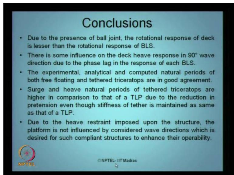
So, some quick conclusions from this what we are shown you are due to the presence of ball joint, the rotational response of deck is far lesser than that of the BL. There is some influence on the deck having in heave response in 90 degree, which can be due to the differential phase lag of different BLS because they are independent to each other, the experimental, analytical and computed periods closely agree.
