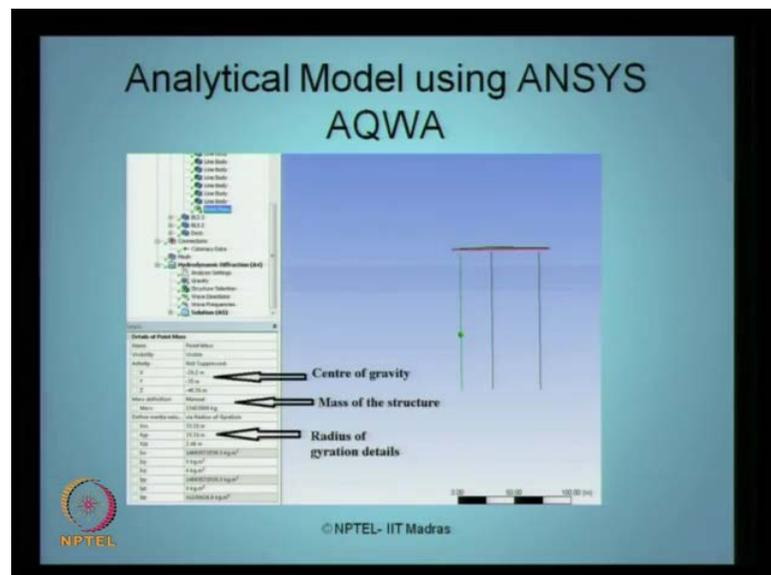
Once this is done then you have to specifically enter the values of centre of gravity, mass of the structure and radius of the gyration, which can calculate mathematically once you know the  $M$ ,  $r_x$ ,  $r_y$ ,  $r_z$  values for the given geometry. So, this is what, we entered here so
