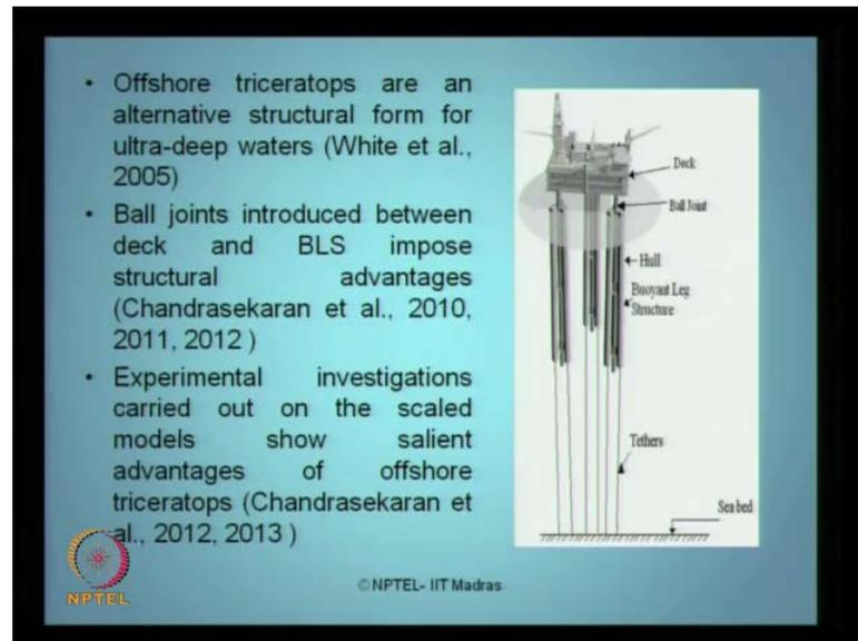
So, the third structure is what, we have originated in our studies here, which is again a concept of triceratops. The triceratops concept was first floated white et al 2005 and he said, yes this platform can be used comfortably for deep water oil exploration. Because, there are some structural advantages, which this platform has let us see, what are the advantages quickly, as we go through this presentation?
