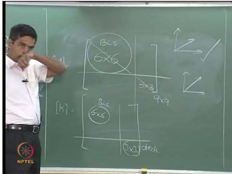
By mass matrix, I am partitioning it, this is 6 by 6 and this is 3 by 3 so I have the mass matrix of 9 by 9, this corresponds to BLS because in the cg of BLS, I have all the degrees present. Corresponding to the deck, I have only 3 degrees present, which are only the rotations because the rotation of the deck are the independent of that of the BLS. But, the displacement degrees are common in both cases, because of rigid body motion so easily I can find out the mass matrix of the sub structure.
