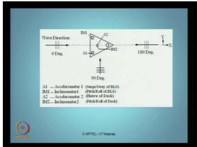
This is my wave direction so therefore, you can see the instrumentation on the top for the experimental analysis, accelerometers of A 1, etc has been kept. One on the cg of the depth and one on the one of the BLS to compute the relative motion between the BLS and that of the decks independently. They are all tri accelerometers, which can measure the surge and sway depending upon, what you want and inclinometer will give you the differential rotation.
