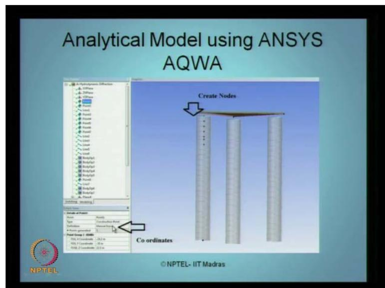
Interestingly, a numerical study was also done on this platform using ANSYS AQWA, I will show you some steps, as to how this ANSYS AQWAA carried out. So, in the first step, the coordinates were introduced by creating nodes, these are the coordinates manually given as an input in ANSYS AQWAA to create the nodes.
