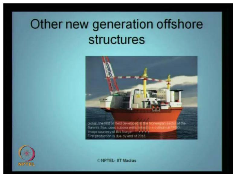
The other one is again a non ship shape of course, a circular hull is called a goliath, it is the first oil field developed in Norway sector, is a cylindrical FPSOs. So, the production is due by end of 2013 again, again a ship shape FPSO non ship shape FPSO.
