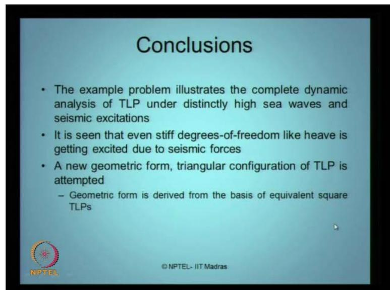
The example problem illustrates the complete dynamic analysis of TLP under distinctly high sea wave seismic excitations. We can see this from the example even the stiff degrees like heave is getting excited because of seismic forces. Distinctly, a loop
