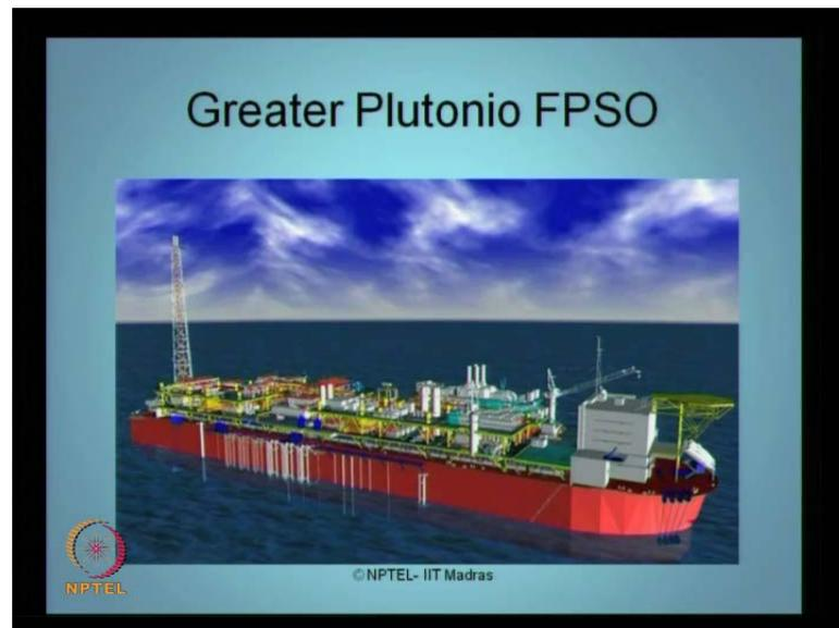
So, they can be as large as it is about 183 meter long 62 meter wide. It is very long FPSO; generally these are all existing vessels being converted for this kind of purposes plutonio is a very famous FPSO being commonly deployed. We will quickly look at the mooring and station keeping, because we were do when orthoflex analysis, later in the next module.
