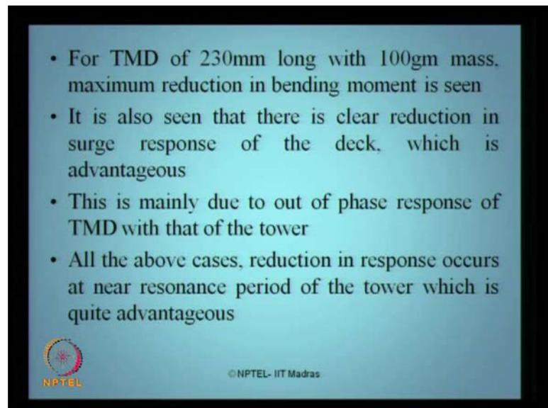
So, for a T M D of 230 mm long with 100 mm gram mass, the maximum reduction of the bending moment is seen. It is also seen that there is a clear reduction in the surge response of the deck for about 10 percent, which is advantageous. This is mainly due to
