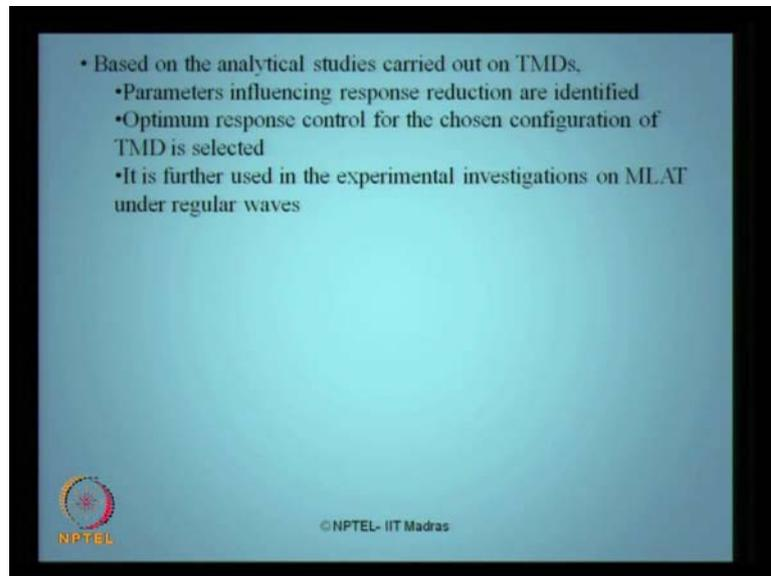
Now, let us see how this experiment was conducted? So based on analytical studies carried out the optimum different ratios of secondary mass to the primary mass system, that's why we call just tuned mass dampers. I got to find out, which mass proportion of  $\mu$  will comfortably work at the bandwidth of  $(\sigma)$  frequency the wave from which chosen fundamental frequency  $\sigma$ .
