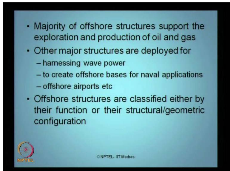
The majority of offshore structures support the exploration and production of oil and gas platforms the other major structures are generally deployed other than for oil exploration or essentially for harnessing wave power because we have got floating devices where people start installing it on the floor on the sea wave to harness wave energy.
