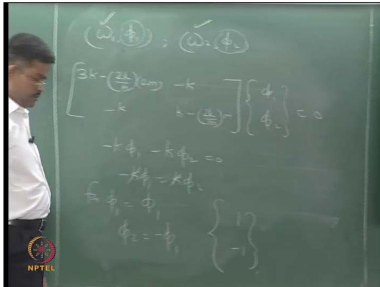
So, for every frequency there is a corresponding mode shape; for every frequency there is a corresponding mode shape. I know these two values, I do not know them, I am interested to find out this. So, if I really wanted to know phi 1, I must substitute here. Instead of omega I should say omega 1 and get phi 1; if I substitute omega 2, I will get phi 2. So, corresponding values, this cannot be pair decoupled, they are pairs and this combination is unique.
