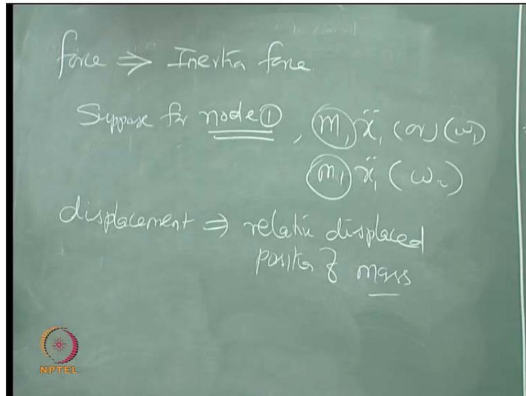
We are talking about some force, what is that force because we say, that deflection at mode two, we are talking about forces, the force what we refer here corresponds to inertia. Suppose, suppose if you take node 1, node 1, that is, node 1 if you take, node 1 you must apply,  $m_1 \ddot{x}_1$  or  $m_2 \ddot{x}_1$ , corresponding to either  $\omega_1$  or... You must apply  $m_1$ .
