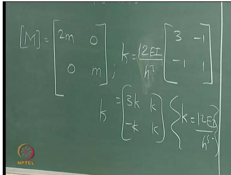
$$[M] = \begin{bmatrix} 2m & 0 \\ 0 & m \end{bmatrix}; \quad k = \frac{12EI}{h^3} \begin{bmatrix} 3 & -1 \\ -1 & 1 \end{bmatrix}$$
