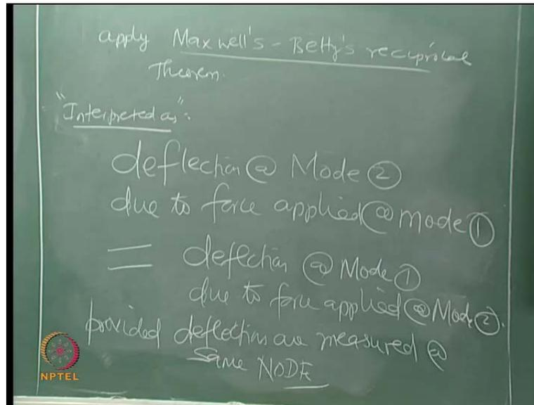
Now, one may ask a question, that why orthogonality is important? The moment this mode shapes becomes orthogonal, then the advantage starts from applying, you can apply the Maxwell's-Betty's reciprocal theorem directly to this problem if the mode shapes are orthogonal. Now, what is Maxwell's-Betty's reciprocal theorem on dynamics? Because this theorem is on statics, statistics, how this theorem can be applied to dynamics?
