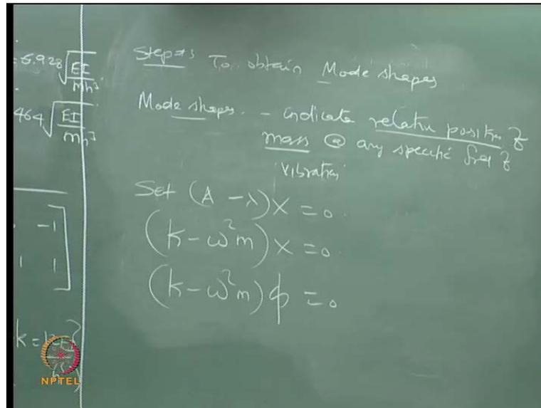
So, step number three, to obtain mode shapes. Now, what are mode shapes? Mode shapes actually indicate the relative position of mass at any specific frequency of vibration. For example, if the structural system is vibrating at a specific frequency of  $6.928 \sqrt[3]{EI/mh^3}$ , then what would be the relative position of the mass points in the given system? If I try to plot that graphically, that is what my mode shape is, so I want to find the mode shape now.
