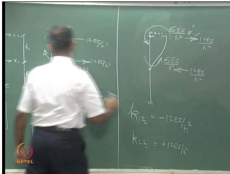
Let me give  $\delta$  here, so this is going to cause a moment, which is  $6EI$  by  $h^2$ . Of course,  $\delta$  is unity, I am putting here  $I$  because this is only  $k$ , the stiffness is only single, whereas this is  $12$  because this was  $2k$ , so this is an anticlockwise moment of  $12$ . So, there is going to be a couple, which is  $12EI$  by  $h^2$ . So, I am going to derive now  $k_{12}$  and  $k_{22}$ .
