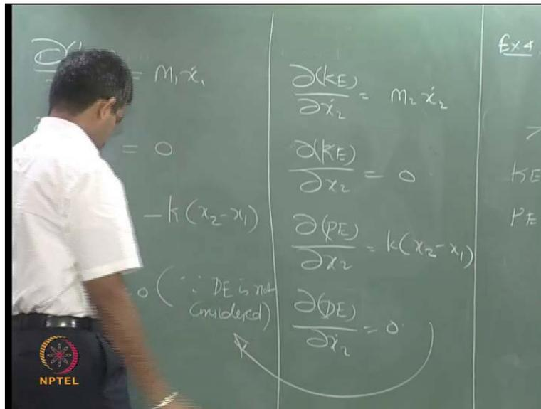
Similarly, I can do for the second case. So, do kinetic energy by do  $x_2$  dot is  $m_2 \ddot{x}_2$  do kinetic energy by do  $x_2$  is  $k(x_2 - x_1)$  do dissipation energy by do  $x_2$  dot is set to 0, because of the same reason.
