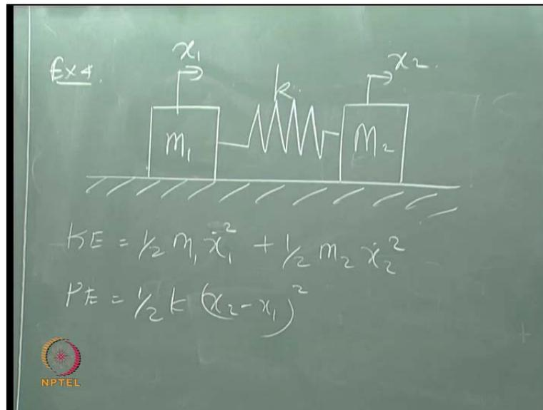
So, we will neglect the frictional forces between the mass and the contact points. So, kinetic energy, half  $m_1 \dot{x}_1^2$ , that is, half  $m_2 \dot{x}_2^2$ ; potential energy, half  $k$  relative displacement. So, we will use Lagrange's equation to write down the equations of motion based on energy method. The Lagrange equation says, first find the partial derivative of the kinetic energy with respect to each one of the degree of freedom.
