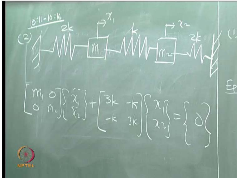
So, I want you to quickly write the equations of motion for the second problem, which I am giving here. I will give you five minutes time. So,  $m_1$ ,  $m_2$ ,  $x_1$ ,  $x_2$ ,  $2k$ ,  $k$ , so the equation of motion is given. This is how it is obtained. Let us do one more problem. I want you to write the equations of motion for this problem.
