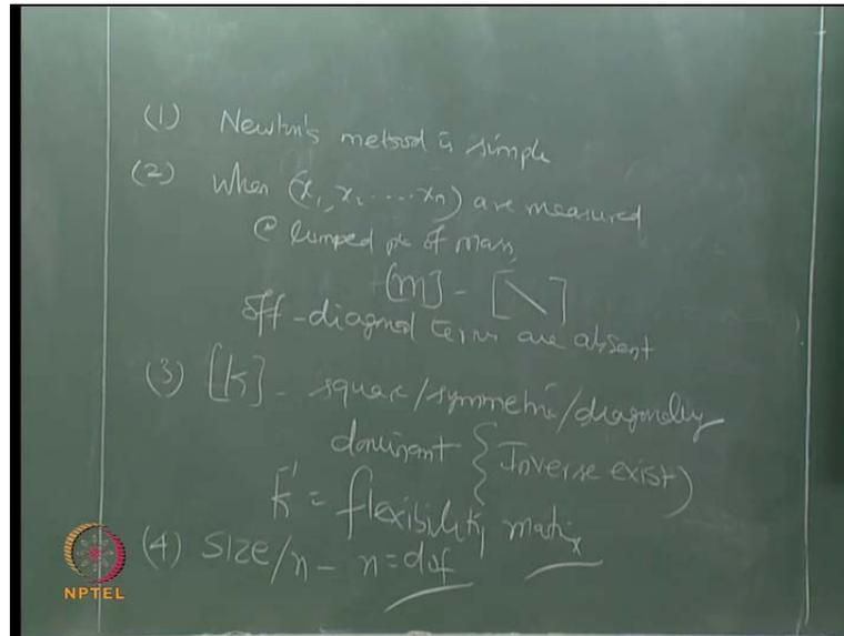
The first information I derive is writing equation of motion. For a two degree or multi-degree, using Newton's method or Newton's law of motion is simple. I can also use energy method, I will show that later. The second inference I derive is when the displacement coordinates are measured at lumped points of mass, mass matrix becomes diagonal. It means off-diagonal terms are absent.
