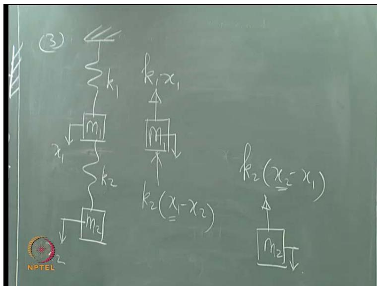
I can draw a free body diagram. I am helping you, if this mass moves down this spring will try to restore it back. So, this will be  $k_1$  of  $x_1$ , whereas this spring will try to push it up. So, it is going to be  $k_2$  of  $x_1$  minus  $x_2$ , that is, for the mass  $m_1$  and so on.
