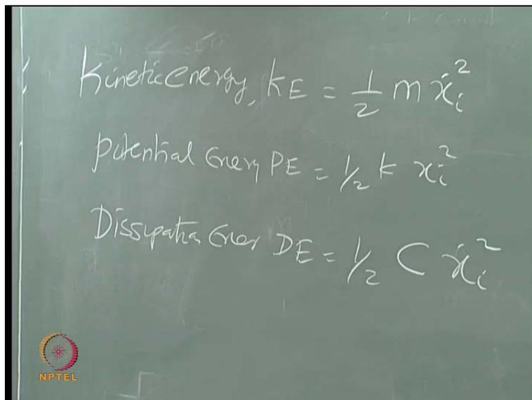
Whereas, kinetic energy, potential energy and dissipation energy are given by the following equations: kinetic energy, half  $m \dot{x}^2$ ; potential energy, half  $k x^2$ ; dissipation energy, half  $c \dot{x}^2$ . So, use these expressions now and let us try to write the equations of motion for a two degree freedom system, as I am going to show you now.
