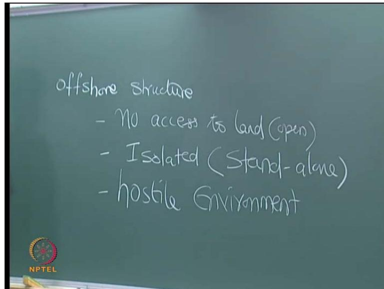
So, foremost condition for an offshore structure is? For any offshore structural systems, the foremost requirement which is dangerous is, it has no access to land which is openly available. So, they are isolated; what we call them as standalone systems. They are subjected to hostile environment. In case of any correction, any repair or any emergency, you want to attend but they are not readily accessible. So, this limits the number of installations to be very less.
