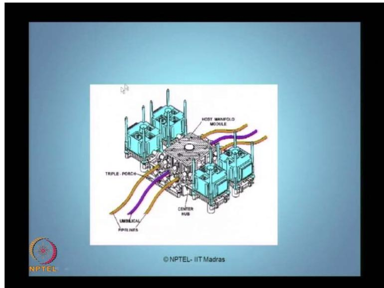
We can see a typical figure of a template which contains umbilicals. Umbilicals of given different color; this can be either different conduits, can be even pipes, can also have what we called pipelines which are given in different color. We have center hub, which connects the host manifold module to that other different facility.
