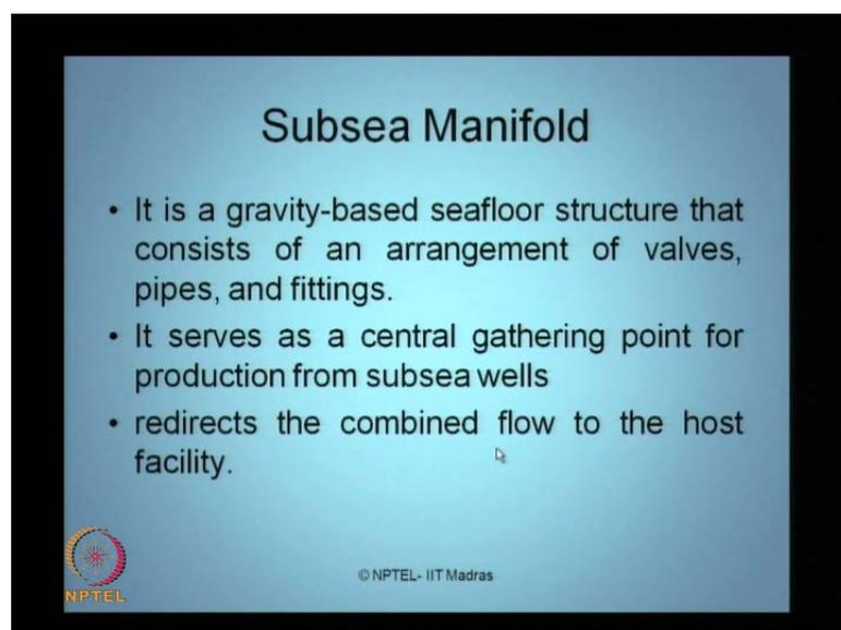
Let us talk about another important component of the subsea system, which is subsea manifold. What is the subsea manifold? It is actually a gravity based seafloor structure.
