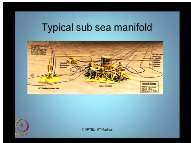
This is the picture, which shows you a typical subsea manifold as you see here. The manifold is connected to 12 inches flow line laydown sled here in the side. As well as the different umbilical cables which have been connecting the flow line laydown the subsea manifold. As I said if it is localized, it is a flow line; if it is spread wide for a longer length, it may be a pipeline.
