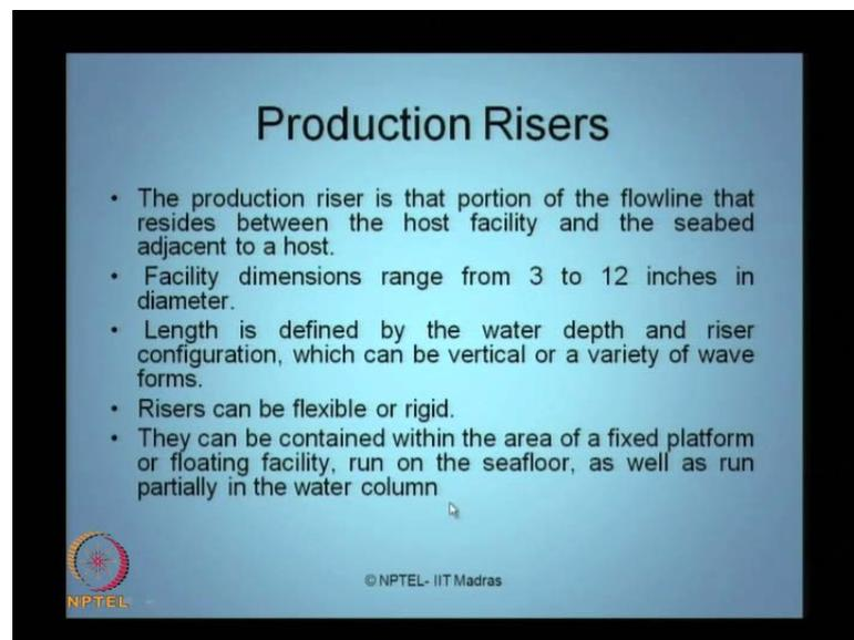
Let us talk about another important component of a subsea system, which is production riser. The production riser is that portion of a flow line, you must understand what you mean by a flow line; it is different from a pipeline. The production riser is a part of the flow line that is located between the host facility and the seabed adjacent to the host. Host facility can be any one of the types of platforms, which we have learned by this
