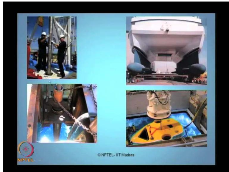
These are some of photographs which show you the details of moon pool. You can see here moon pool is nothing but hole, which is driven the top of the hull which passes through and through. You can see here the hole through and through, you can see the waterbed here, and you can see the sea surface here. This is the very specific drilling mechanisms or the drilling risers are connected in pieces has the drilling progress deeper and deeper.
