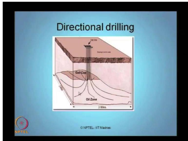
What you understand by directional drilling? Ladies and gentlemen, as you see here in this figure, if you want to do a drilling actually from the moon pool of a ship. I said the moon pool should be located exactly above the drilling hole, I prefer to drill vertically down, but sometimes we have to also extend the drilling not exactly vertical but also have possible lateral direction to touch as far as possible the boundary of the hydrocarbon traps.
