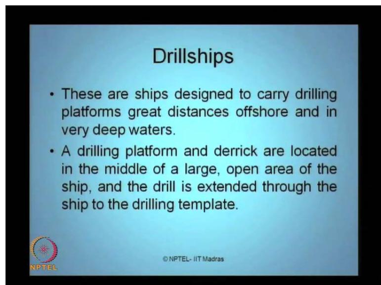
Drills ships are designed to carry drilling operations are greater distance offshore and in very deep waters. A drilling platform and derrick will be located in the middle of a large, open area of the ship, the remaining recollect terminology which is middle, large, open area in the ship which a called as a moon pool. Moon pool is nothing but is hole extended through the hull through which the drilling rises will be placed through the hull to the drilling template.
