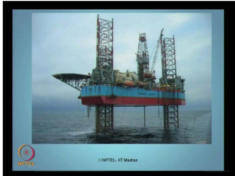
You can see a closer view of a jack up rig which is masks giant; it is the top side. The red (( )) you see here is actually an index; for us to understand, it is a maximum water level. Now, you can see, the three lattice legs which is coming out from the tower; you can see a helipad which is being used for helicopter landing. You can see a very complicated top side facility is being given, or made available on these jack up rigs.
