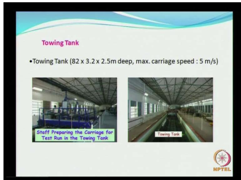
So, this is something to do with the theoretical spectra which I will not cover this; there is in addition to the wave flumes we also have what is called as a towing tank as we have as I have mentioned earlier basically to the dimensions are given here. Basically to measure the resistance of the ship motion - ship models, and other related test related mostly related to ((C)) engineering.
