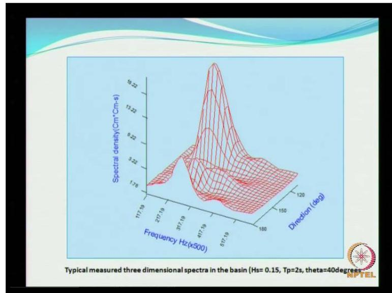
This is a typical directional spectrum which we have measured. So, you see that this is the energy distribution, this is the spectral density which you know and this is the energy, and as a function of frequency, and also as a function of direction. So, if you take one direction you get one spectrum or if you take one frequency you will get the distribution of energy as a function of direction. So, that is what it gives the directional spread.
