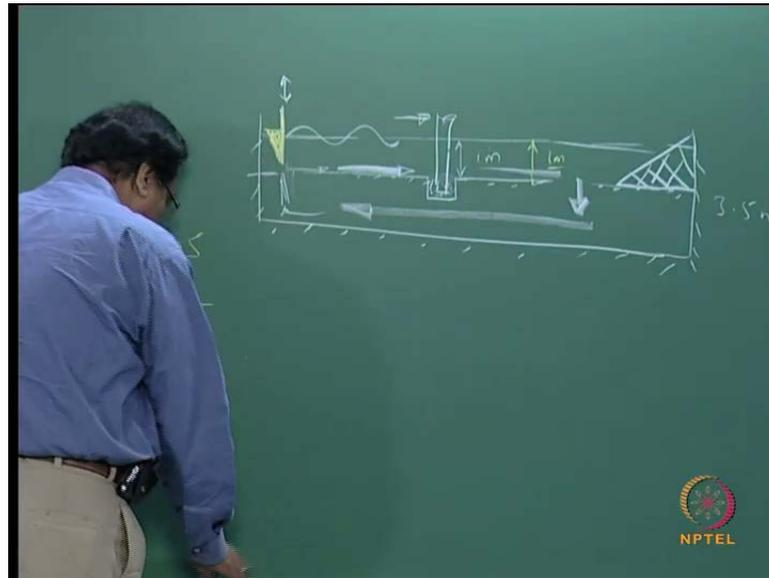
So, later you will see that we **we** will see the cross section of the flume, wherein under since the flume **is** was three and a half meter **long** deep. What we decided was to have a false bottom, and so that the water depth now in this case will be around one meter say. So, this bottom of the flume will serve as a reservoir for you have a suction pipe; the water will be sucked in with a motor and the delivery will take place here.
