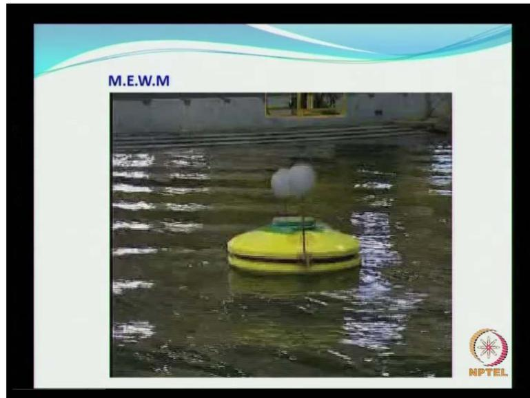
And then we just move on to the multi element wave maker. Now, you see that all the single units of 52 in number, the number of units are moving in unison that is as a single piece. So, generating long crested waves, that is what can be generated with the long crested wave maker; it is the same model that is being tested here.
