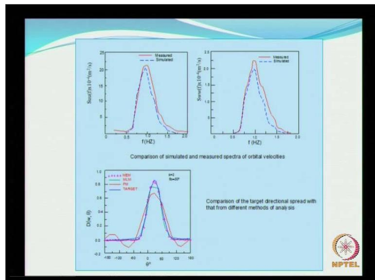
And then these are showing some of the typical comparison between the measured and the simulated target spectrum. I think this is for the orbital velocity for the same time histories, which we saw the comparison between the measured, and the simulated orbital
