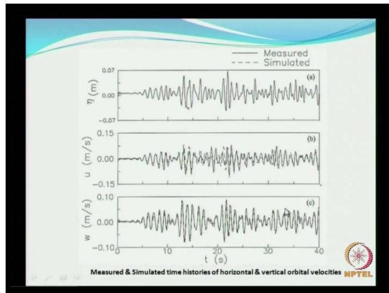
So, here in this is a typical result which we have got obtained from the wave tank test, this is the simulated wave for which you have measured and simulated particle velocity in the horizontal direction, and in the vertical direction just to prove that your measurements and the simulations.
