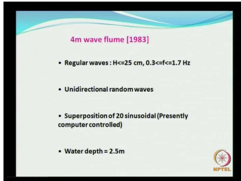
Now, the 4m wave flume, this is 4 meter wide wave flume; it can generate regular waves up to about 25 centimeters, then the frequency range is similar to that of the older flume wave maker and it can generate only unidirectional random waves. You can generate of course, when I say random waves it is also it also includes regular waves.
