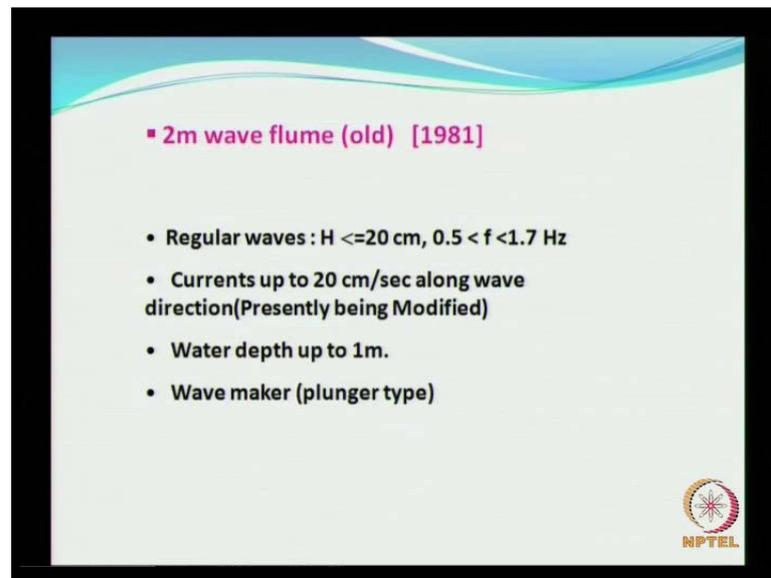
So, initially we had a 2 meter wide wave flume 30 meter wide; and the depth of the flume was 3.5 meters, with a wave maker on one end; a simple plunger type wave maker which can move up and down; and based on which it can generate waves height up to about 20 centimeters; and the frequency was ranging between frequency of the waves that could be generated in the flume varied between 0.5 and 1.7 Hertz.
