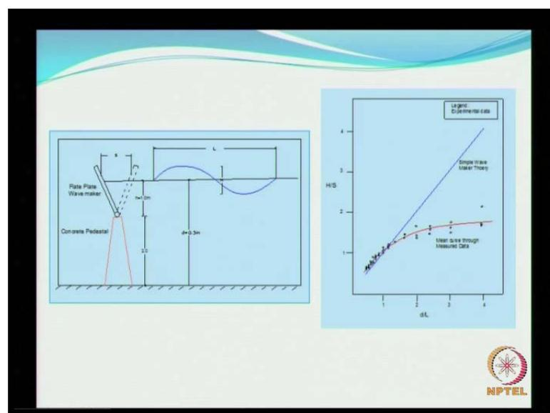
It is mounted on a pedestal here, it is 2.2 meters from the floor. And then you have 2 meters from the floor, and then you have the wave maker here moving that can be moved, and then you can generate the waves. And these are the information concerning the maximum wave height that is this is the simple wave maker theory, that can that gives you the wave height that can be generated by the wave maker theoretically.
