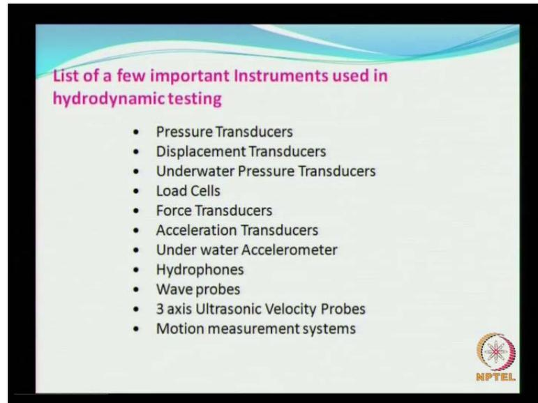
**List of a few important Instruments used in hydrodynamic testing**
