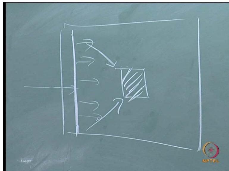
One way of testing the oblique waves is, that you have a basin you have a basin and you have a wave maker. This is not; I am not talking about multi element wave maker. It is a simple unidirectional it can generate only unidirectional waves. For example, then in that
