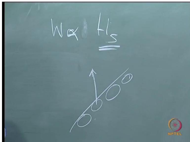
The effect of wave groups is, suppose, if you are designing a rubble mound structure. The weight of the individual stone is based on weight of the stone is directly proportional to  $H_s$ . So, assume that you have designed the stone and there may not be a problem, if wave height is slightly exceeding even the  $H_s$ , once in a while it does not matter. But very frequently it exceeds the significant wave height. Then, what will happen? That is
