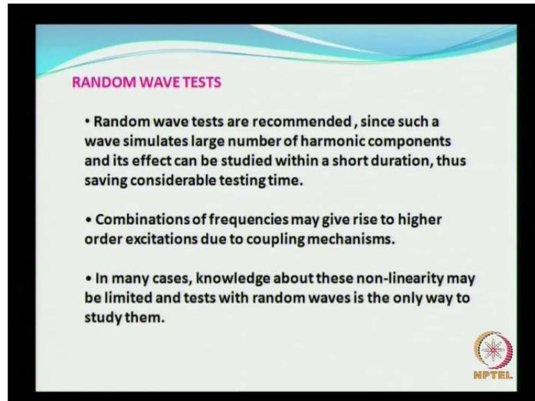
Now, random wave test. Why are we talking about random wave test? Random wave tests are recommended, since, such a wave simulates large number of harmonic components and its effect can be studied within a short duration. So, thus saving considerable testing time, this is also very true.
