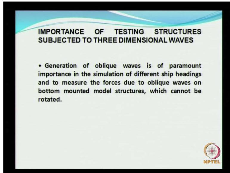
Then in continuing the oblique wave, generation of oblique waves is of paramount importance in the simulation of different ship headings. And also to measure the forces due to oblique waves on bottom mounted structures and in which case the bottom structures, bottom mounted structures cannot be rotated.
