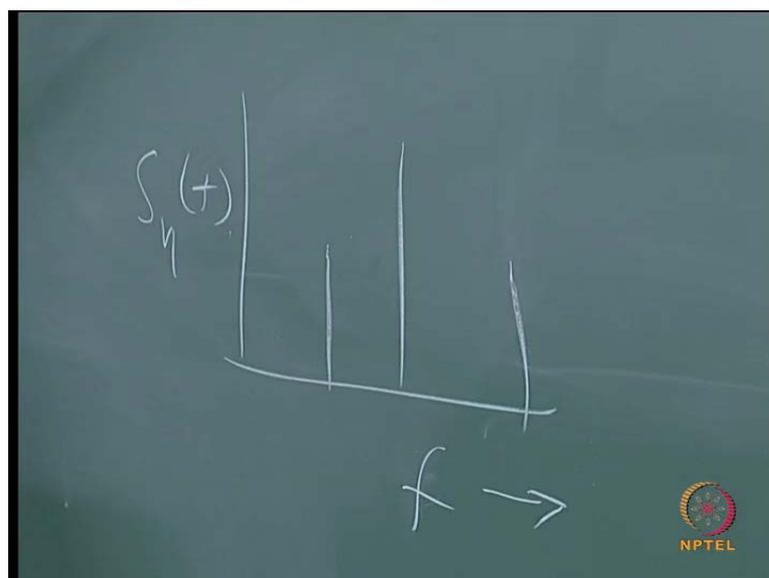
Then, I can get some kind of a frequency response, frequency the spectrum. Where in, on the x axis I will have frequency, on the y axis I have spectral density for example, or heave response function.
