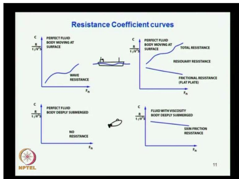
So, this are representation of a resistance coefficient we say different you know cases when you can say that fluid, here you consider perfect fluid body moving at surface. So, you consider a perfect fluid means there is no viscosity and the body is at surface. So, there is no frictional resistance, only the wave making component. So, you can say that
