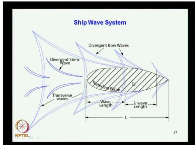
This is another systematic representation of that ship base system, we can see the ship waves are generated and they give this a divergence wave is coming out. And these waves which tangentially you know join at you know, which get such a shape converse shape here this is called the transverse waves. And these waves systems are generated from different regions of the ship, you can say that starting from here another system from here another from here another wave system from here.
