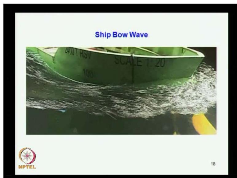
I can see in this slide, see the it is the model test which is been carried out here in the institute. You can see that the wave elevation at the bow part here I can say the height is more compared to other region. So, that is called the bow way, the wave formed at this part. So, when this wave go beyond the height the wave would not be able to retain its
