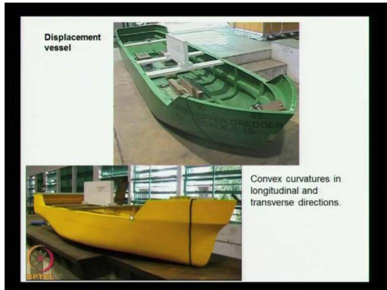
We can see that it is the shape you can see the transverse is convex and also you say longitudinal also, it is a convex shape. So, you can say that this is a displacement vessel which is having a convex curvature in the longitudinal and transverse directions. So, the convex curvature in the longitudinal and transverse directions, this reduces a flow separation at the stern and bilges. So, a smooth curve a convex curvature reduces that flow separation because it is a smooth shape.
