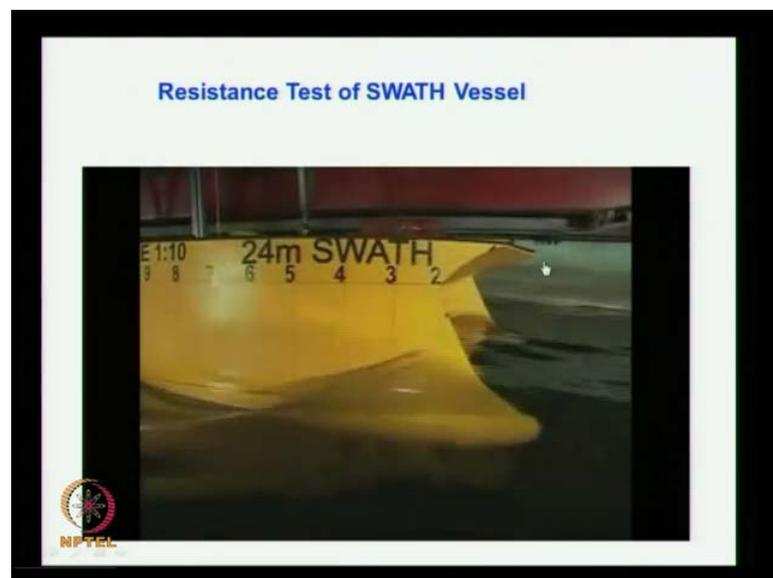
We tried different version of the and also different configuration of the Swath vessel and the you can see here in the middle there is a gap. This is actually 4 hulls 1 hull 1 hull here another hull here the same thing on the other side. And you can say the middle
