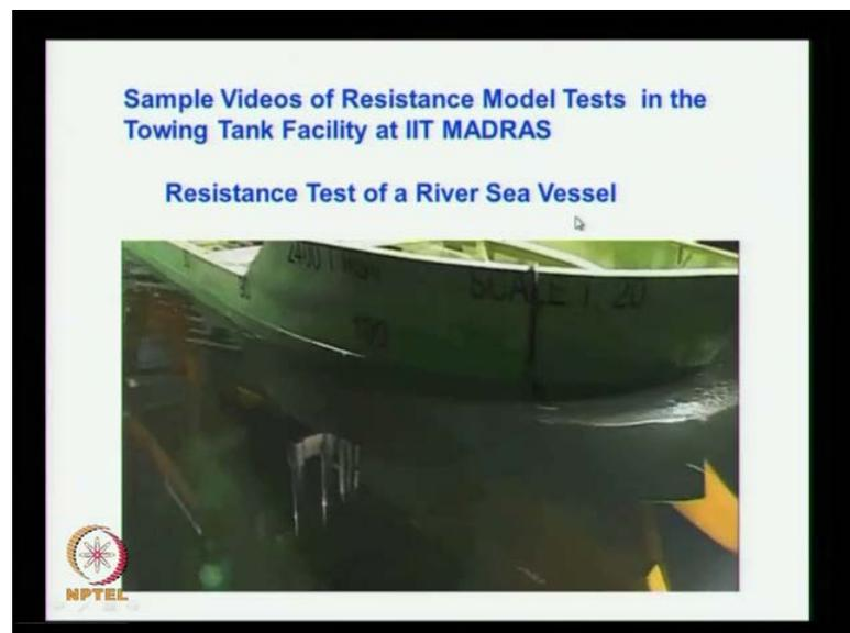
So, this gives you can see this test not only resistance. It also gives the pattern of wave around the vessel you can see that pattern of the around the vessel from the video or form the observation. If you find out the wave is going to be high and the wave makes resistance high you will get an information which art of the ship is creating more wave. And where you need a attention to modify the form that region, so that wave making
