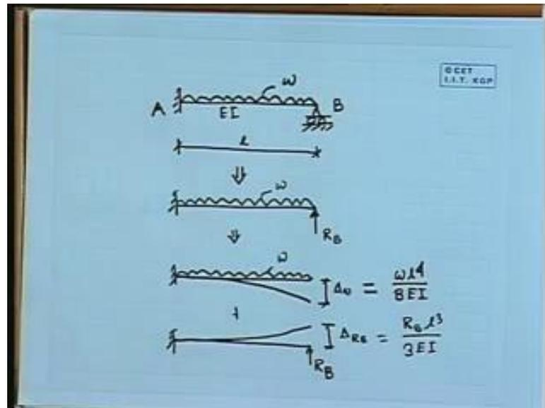
Or if I take the cantilever problem; cantilever problem we have removed that. Here, the restrain against rotation we can release. So, we can make it simply supported. So, we can make it a hinge support, with a applied load, and that load will be in the form of your bending movement. So, one bending movement will be acting at the end and that bending movement is a unknown quantity. So, it will be simply supported beam, fully loaded, plus a end moment. So, one extra quantity that.
