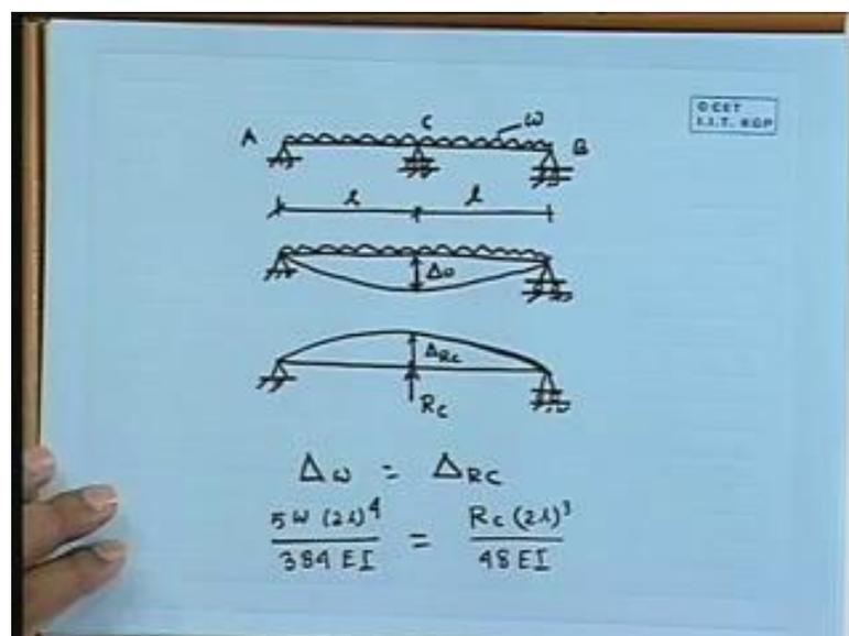
So, if we come to the original problem. So, here this was removed by a force; we could keep the support; remove this one; and put a reaction here. That can be also done or we can keep the support, remove that, put a reaction there.
