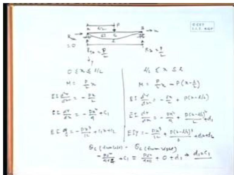
Say here; here to here  $M$  equal to  $P$  by 2 into  $x$ ; and here to here it is, say, this force into  $x$  that part is there, minus  $P$  into  $x$  minus  $l$  by 2, because here if it is  $x$ , so  $l$  by 2 minus that is the distance  $P$   $l$  minus  $x$   $P$ ; that part it will give a hogging moment, and this part will give some sagging moment.
