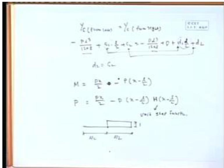
Y at c, it is from left YC from right. So, here we have the equation it will be minus pl cube divided by 12 into 8 plus C 1 l by 2 plus C 2; it will be equal to minus pl cube 12 into 8. Incidentally, that term will be equal to 0; the additional term what you will get at that point plus D 1 already we have obtained it is equal to your C 1 it is l by 2 plus D 2.
