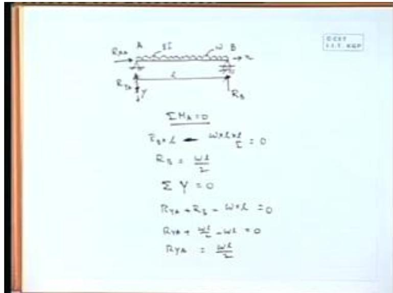
So, this is a distributed load of intensity omega or w; and the member is some EI; the flexible rigidity; this is the length; this is x this is Y. So, our first job is to determine the expression of bending moment. Now, if we start from this end or the other end, both the sides supports are there. So, we have to know the value of those reactions.
