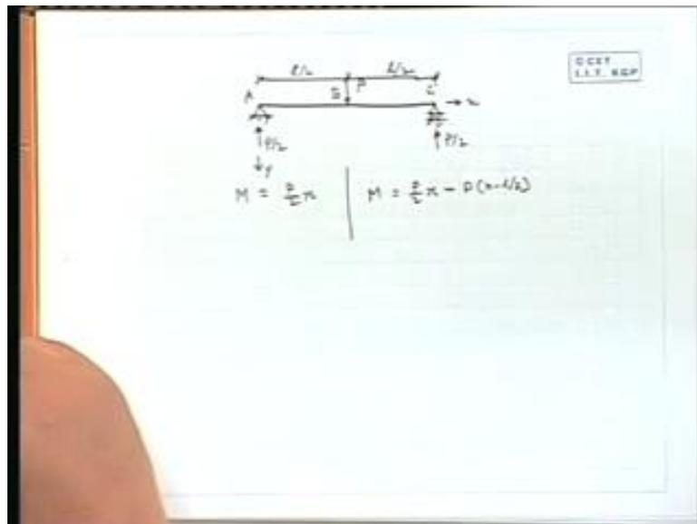
So, we took a beam like this this side some support here also, we support and centre we put P reaction we got P by 2 reaction P by 2 if we say this side is x that side this is y.
