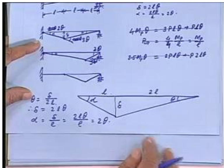
Say, this angle is alpha; this angle is theta. Let me say this is delta and this is 2 l and this is l. So, what is theta? Theta is equal to delta by 2l. Therefore, we can say delta is equal to 2 l theta. And what is alpha? ((Refer Time: 50:15)).
