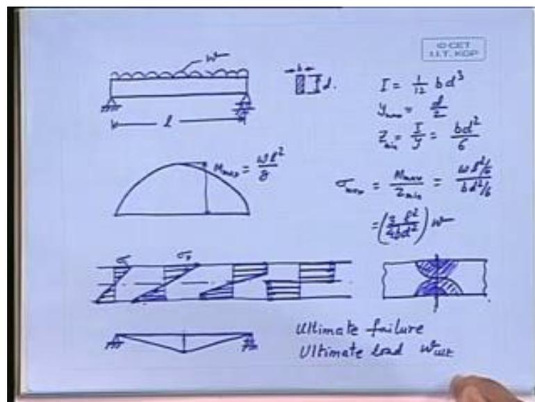
So, if you consider that the material is linearly elastic fully plastic, then let us try to examine a very simple beam and say that how it works in that condition. Say, I take a
