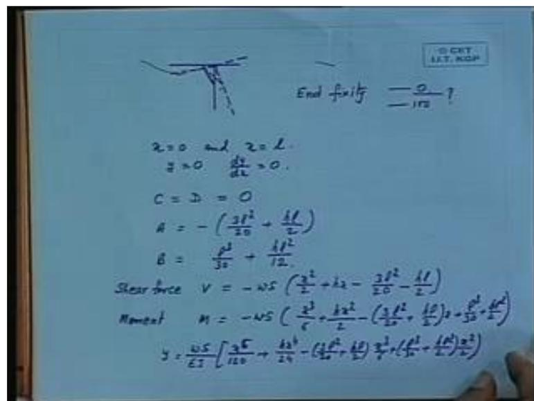
Because of this bracket connection, I am in a position to maintain this 90 degree, but the whole thing can rotate like this because this is in a position to rotate. As far as this connection is concerned, the connection is rigid at that particular point, but as far as the
