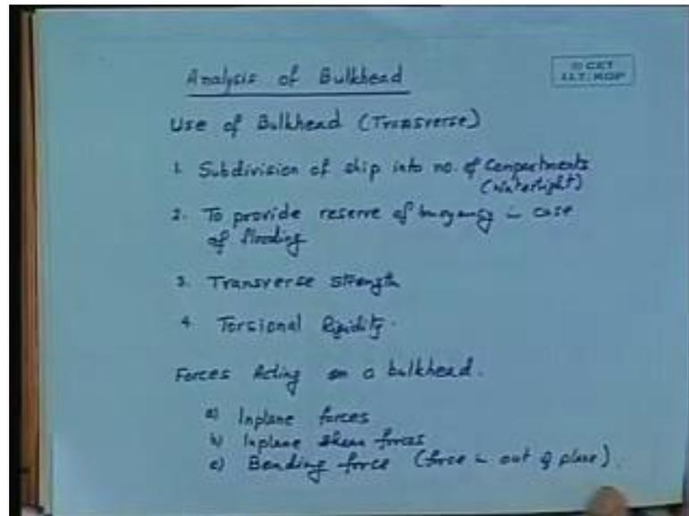
Now, before we go to the topic of bulkhead or the analysis, we should try to understand that why bulkheads are required and once we know why bulkheads are required, then only will try to gauge worth of type of analysis we required. So, let us say use of bulkhead, this can be listed like this number one that when we say bulkhead, it can be transverse bulkhead or it can be longitudinal bulkhead. So, we try to differentiate between the two and we say that transverse bulkhead.
