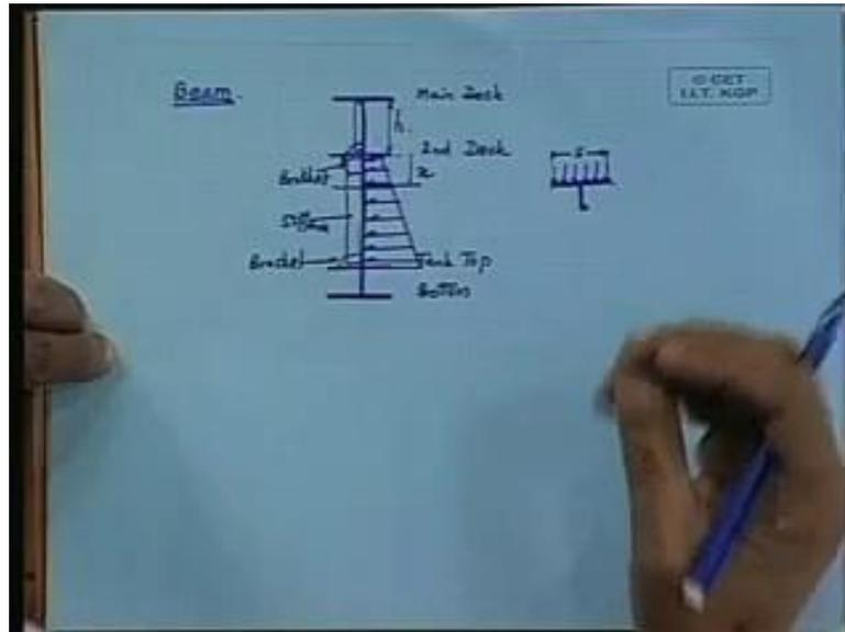
Now, here my primary member is between the second deck and the tank top because the span is more and the load is of this nature. So, we set up, we are considering as a beam. So, from here I set up some coordinate system and I say that my  $x$  is measured this way to some level here, all right.
