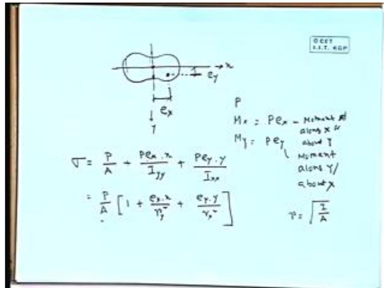
Say if I take any cross section. So, any cross section is quite important here; I will discuss little later, say, this is the centroid or a cross section of a column. Now if the load is acting here, say, this distance we can define it as  $e_x$  and that distance we can write as  $e_y$ , right, say that side if we write  $x$  and this side if we write  $y$ . So, along  $x$  the extensity we are defining as, say, this is the load point. So, this is  $e_x$  and this is your  $e_y$ , right.
