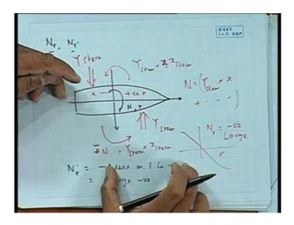
This we understand; now, let us go to the final part - the final part is to find out N r and N r dot; again, we are drawing that and this we will find is going to be...here, according to our previous diagram I have given an r; if I have given an r here - this way - there is a net force y stern; a net force y stem for a positive...we have done that, we have tilted that; as I tilt it this way fluid is pushing this side and pushing this side
