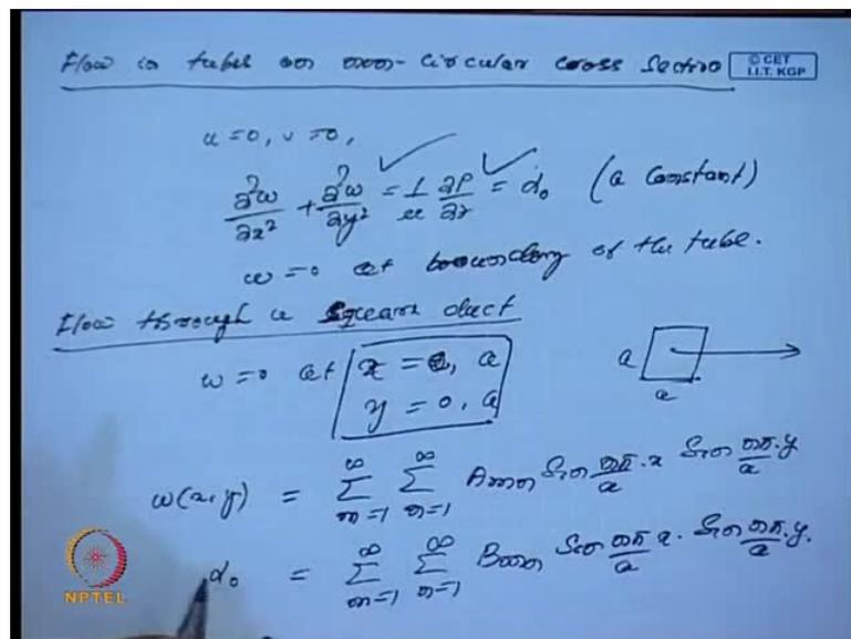
Again I am looking at a fully developed flow, I will have the same thing because a if I recall that I have two dimensional flow, here three dimensional fluid domain and I have a the generator is along the z axis. May have u is equal to 0 v is equal to 0, then I will again another same as assumptions on the for the fully developed flow. I will have del square w del x square plus del square w by del y square is equal to 1 by mu del p by del
