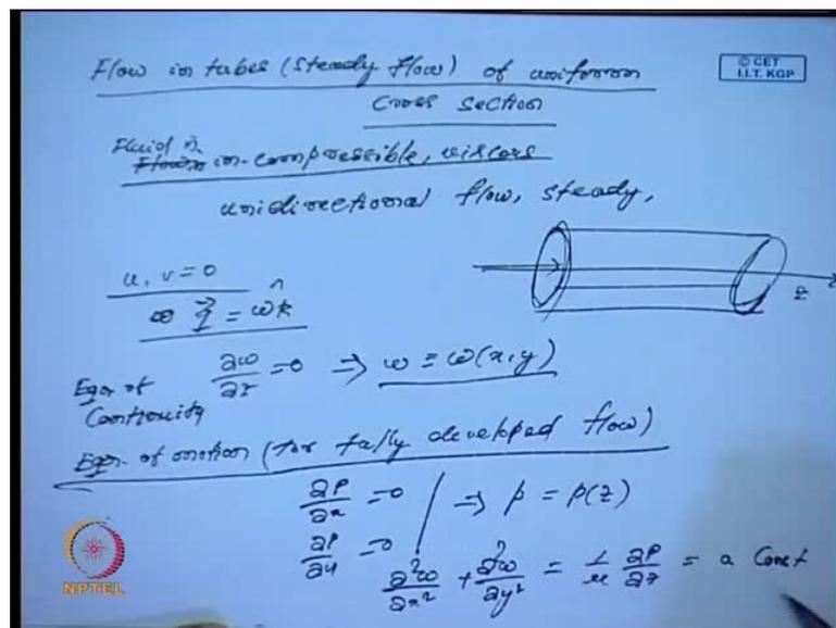
Basically this is a steady flow, flow in tubes of a uniform cross section. So, in this case, I write just, again this are all kind of fully deployed flow, so I will have in the flow is in compression in flow, is in compression, flow is in compression. It is viscous, fluid it is viscous and whether, I will say the fluid is in compressible and viscous and then we have we are considering the unidirectional flow. Assuming the flow is steady, then and I assume that since I am considering a tube.
