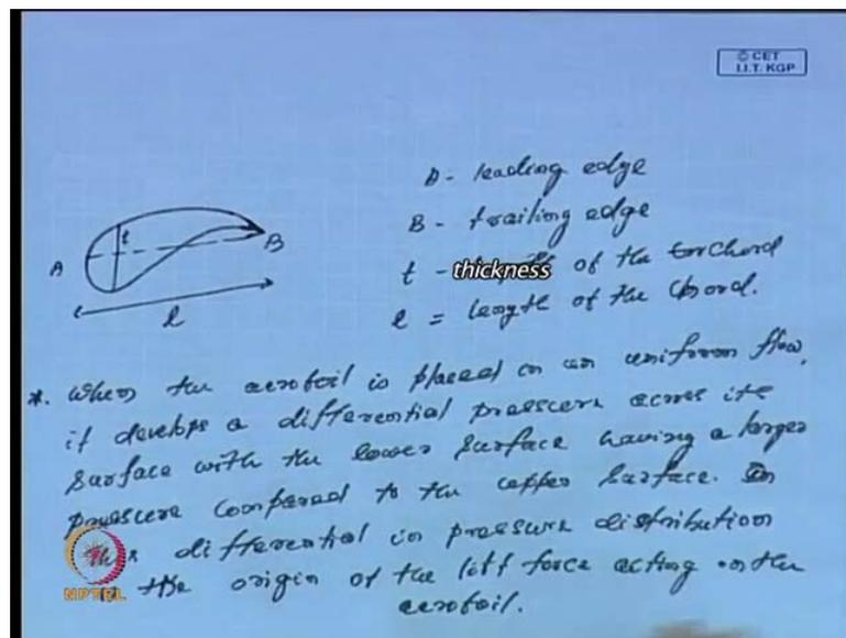
So, if I just consider this, if this is a combined aerofoil, if this is A, this is the B, this thickness that is called t. So, it call A as the leading edge, B as the trailing edge, these are some of the common terminology and t is the length of the chord and then we have l length of the chord. Now this is a some of the common terminology of this section aerofoil section.
