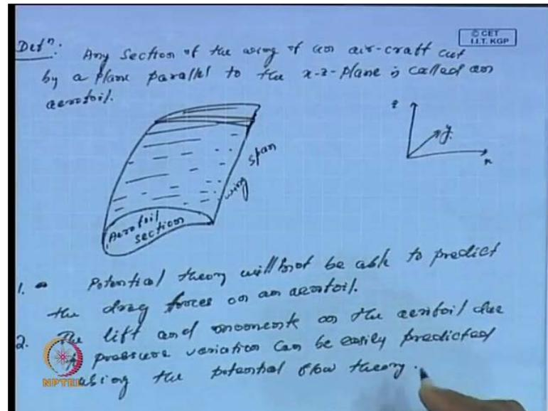
So, while think of the definition, we will concentrate what is an aerofoil section, it is a section, any section of the wing of the wing of the aircraft any section of the wing of an of an aircraft cut by plane parallel to the  $xz$  plane is called an aerofoil section. So, this is a section, I just say, if what is how you describe the  $xz$  plane, this is my  $xz$  plane and this is the  $y$  direction.
