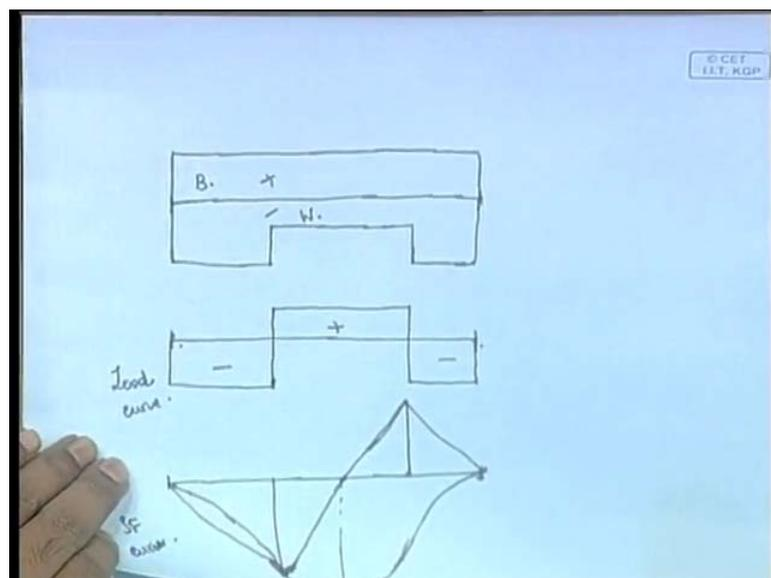
Then, in case of a ship you will see, that so similar to this, we will first of all have or we draw for instance the, the weight curve and the buoyancy curve. In that we have drawn
