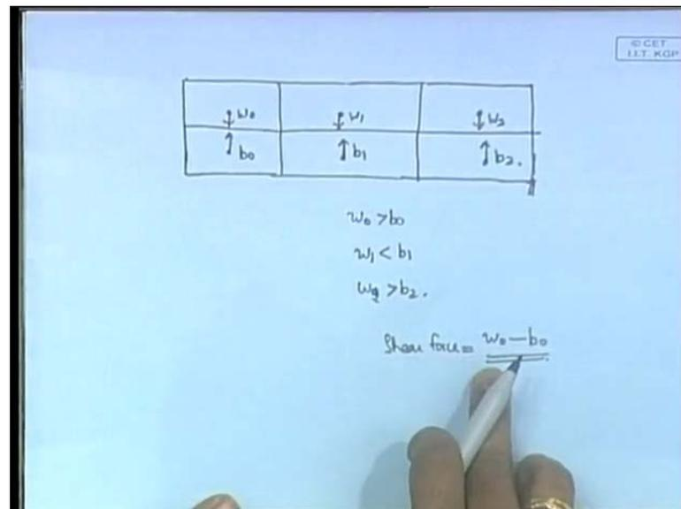
So, we have this, we have this box vessel again. Now, in this case, this is the weight here, let us consider the 3 compartments and let us consider their weights and buoyancy differently. So, this, this is the buoyancy of this compartment, this is a weight of this compartment, then this is the weight of this compartment and this is the buoyancy of this compartment, this is the weight of this compartment and this is the buoyancy of this compartment.
