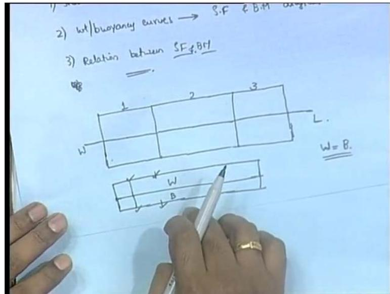
So, now, first of all let us consider a ship like this, that is, we consider a box shaped vessel. Now, suppose, that the ship can be divided into 3 compartments, you have a compartment in the aft, this is the compartment 1, compartment 2 and compartment 3; so, we have 3 compartments. And let us suppose this is the water line, so WL is the water line.
