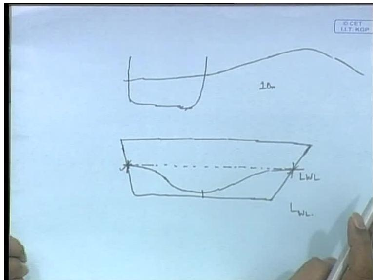
So, if that is the wavelength of the ship, when you are considering the transverse direction like this, which is the breadth of the ship, let us say it is 5 meters or may be even 10 meters. Even if it is a large ship, the breadth might be even 10 meters, so even at distance of 10 meters this waviness may be - it will go like this. It is like this and then slowly goes, so this variation is much larger than, can be seen in a breadth as such.
