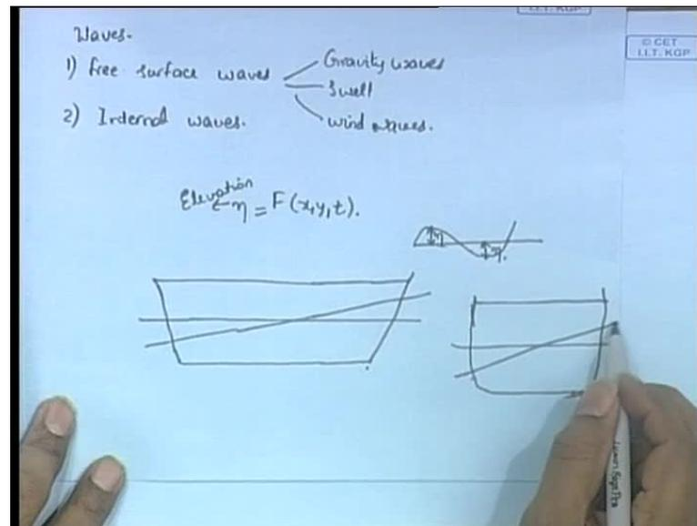
So, we deal with - so there is in naval architecture, a broad category of waves, in which we deal with free surface of the waves. These are the waves associated with the free surface. Then, this is not that important in naval architecture, but in oceanography we come across another types of waves that are associated that are called as internal waves.
