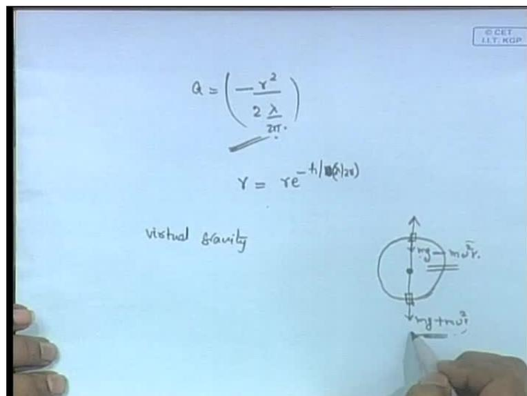
Now, this will be like this, so this particle here it will be subjected into  $mg$  minus  $m\omega^2 r$ , because this will be acting outwards like this. If the particle is at the bottom or other trough, it will be subjected to  $mg$  plus  $m\omega^2 r$ . I hope it is
