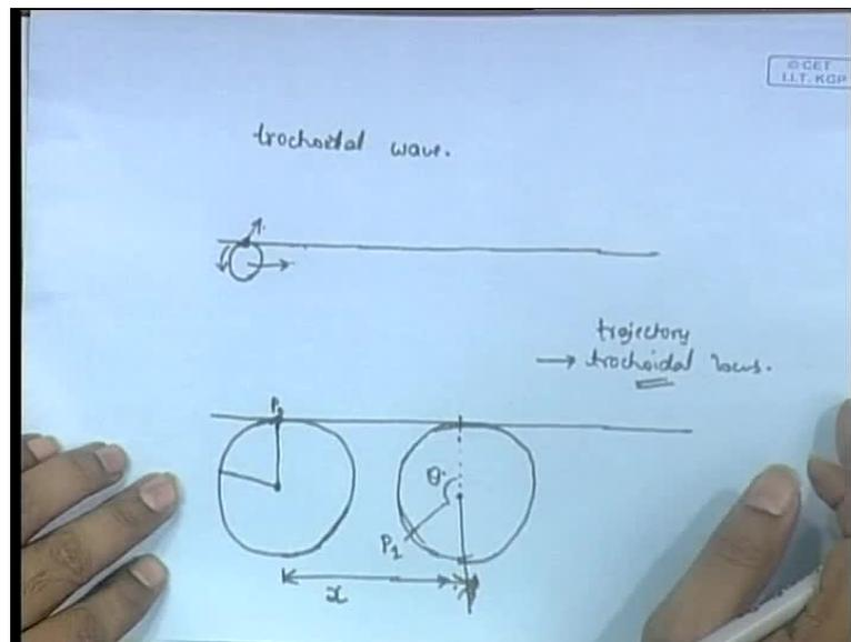
So, if you consider the crest of a wave, in case of the sinusoidal wave, you will see that the crest of the wave is at an equal distance, then the trough in this case also it is true, in trochoidal wave also its true. You will have the crest trough at equal distances from the still line - still waterline.
