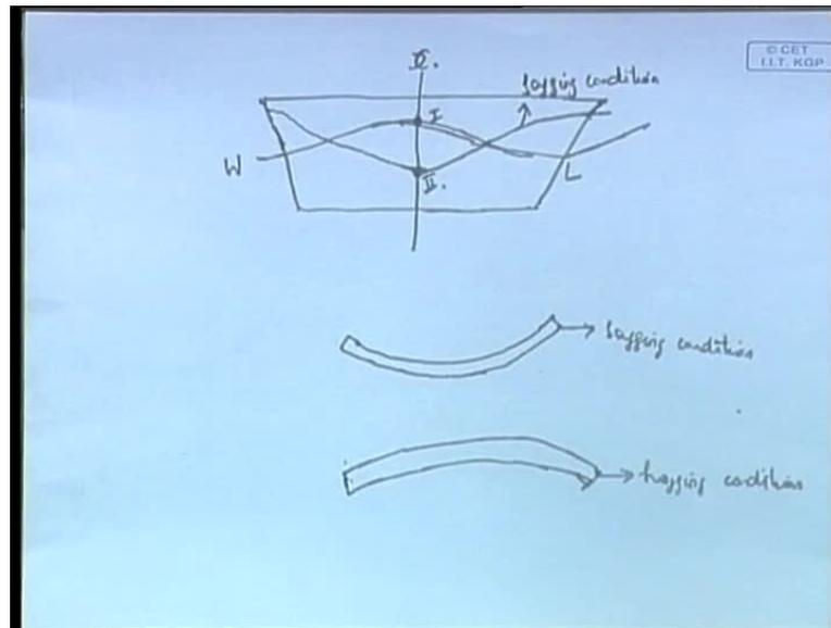
Now, we come to this new type of problems. As I just told you, the presence of waves makes it a curve instead of a straight line. So, it become like this - it become a curved surface instead of a straight line. Therefore, your water line really looks like this, in the presence of a wave, **in a free or** in the presence of the effect of - in the presence of the real free surface.
