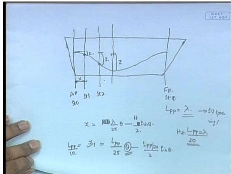
So, like this we have for the first station. Like now, this one, for this particular x, you have this position, so you know what z that we have measured is. This z is actually this; this is the z that you have just calculated. This z means, it is the vertical distance through which the particle has moved, as the result the wave translating a distance x.
