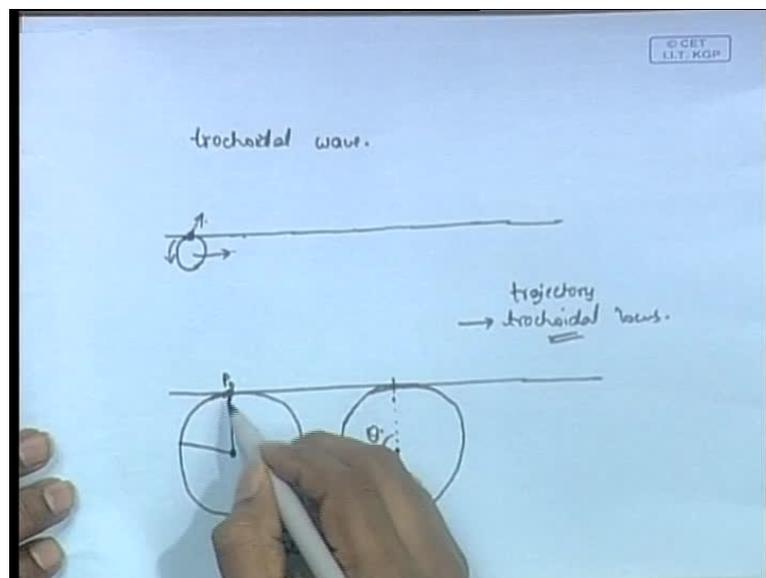
So, this is the circle, this distance is r, therefore this is r, another r, because the particle always goes like this, particle can never move a distance greater than r, because the particle is moving along the circle, therefore the particle can always move a maximum distance of only r from the center.
