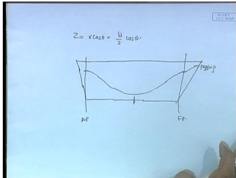
The wave, remember we have define such that you will get - it is defined such that the center of the ship, the midship will have the trough on it. This is L PP, this is the aft perpendicular and this is the forward perpendicular. You have the aft perpendicular and the forward perpendicular, here you will have a crest, here you will have a crest and here you will have the trough.
