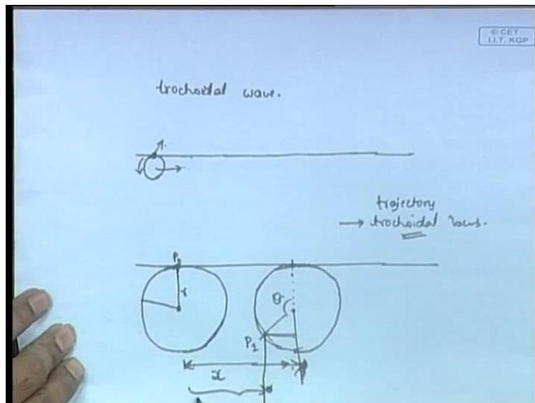
How do you find the position of the - how will you get the  $x$  coordinates?  $x$  coordinates at any center is given by - I mean the  $x$  coordinate of the particle at any point is given by - this  $x$ , which is the distance through which the center of the circle as moved  $x$  minus this distance. We are talking about the position of the particle, note a particle is actually this  $P$ ; it is the particle that is moving along the circumference.
