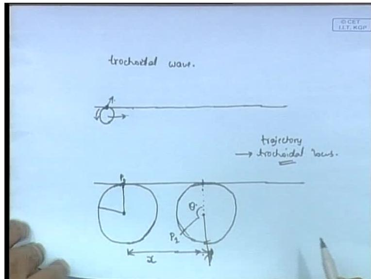
It is mostly in the ocean we consider trochoidal waves. Trochoidal waves; first, before we go into the analysis of the longitudinal section of the ship, we will see what is meant by a trochoidal wave and what is the mathematics associated with the trochoidal wave. This is the - we have what is called as a trochoidal wave, now we will have to define what is the trochoidal wave?
