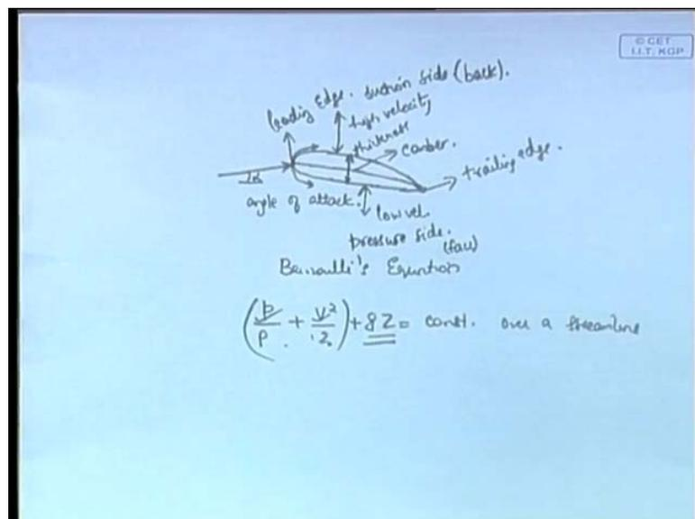
So, we, this is the shape, this is the shape of hydrofoil, now this is known as a camber. This we call it as a camber, the midpoint, the midline, the camber of the hydrofoil, this we call as the thickness of the hydrofoil. So, the camber of the hydrofoil and this is thickness of the hydrofoil. Then, the angle at which, this is a hydrofoil, let us consider
