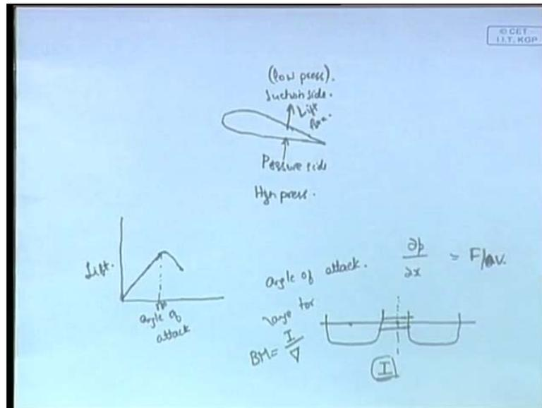
Therefore, you will see that, so if you have the hydrofoil, so this is the pressure side and this is the suction side. So, at the pressure side you have high pressure and at the suction side you have low pressure. So, as a result of which what happens, that is always a force from a region of high pressure to a low pressure. As you know, pressure gradient is the force.
