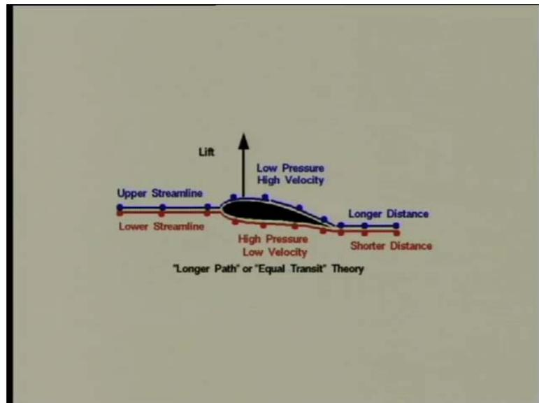
Though not that important for this course, we will just mention quickly, that is, this picture represents how the, this, an example of a hydrofoil or an aerofoil.
