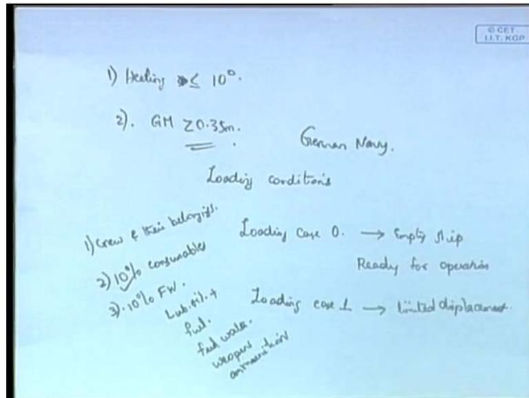
Now, one of the main rules is, that heeling in such small vessels, heeling always does not exceed. That means, it should be always less than or equal to 10 degrees. So, the heeling of such internal water vessels, that is, the vessels in such lakes should always be heeling, should be less than 10 degrees and, and of course, you should have the GM. GM should always be greater than or equal to 0.35 meters, this also holds.
