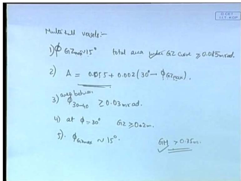
Then, that are some, some kind of rules for multihull vessels as well. So, they, their rules for multihull vessels says, that 1, it says, that if GZ, that is the maximum **righting** arm, is occurring close to the region of 15 degrees, then the total area under the curve, total area under the GZ curve should be greater than or equal to point naught 85 meter radians.
