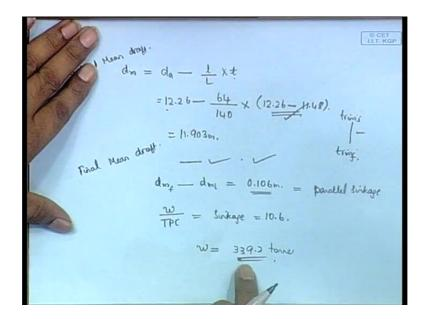
Let us suppose that w is the weight that you are putting in the hold 1.We know that a total weight of 339.2 tonnes has to be added; we have just calculated the total weight that needs to be added. That means let as suppose that w tonnes you are putting in hold 2; that means 339.2 minus w of weight we are putting in the hold 5 - the two holds. As a result of which, what will be the moment? That you have to calculate - that is, I guess the only thing you have to think of in this problem.
