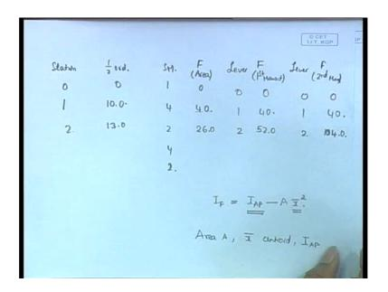
You are given the half ordinates and you are told That means it is like this - for different stations you are given the half ordinates, so we will make the table like this: station; half ordinate; Simpsons multiplier; then you will have a function of area; then we use a lever; then function of first moment; then another lever; then function of second moment - this is to find the this is to find the I F.
