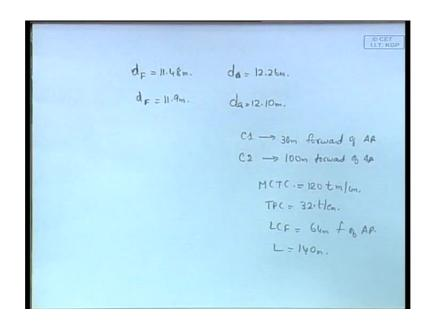
Another problem is - it is told that a vessel is floating at draft forward equals 11.48 and draft aft equals 12.26. Again, actually this is almost the same problem, but slightly different; that is in this it said that finally some loading is done and final drafts are: draft forward is equal to 11.9 meters and draft aft is equal to 12.1 meters.
