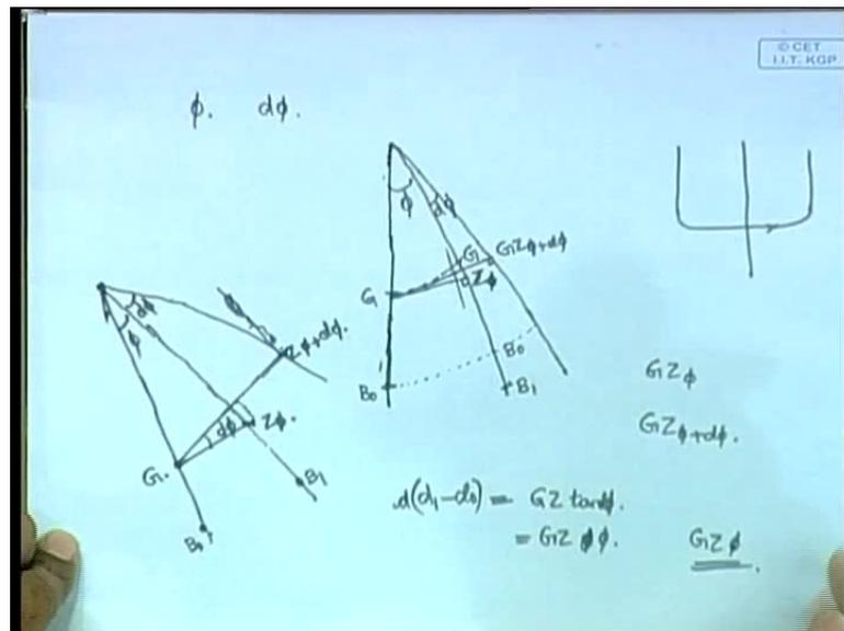
Suppose you have a ship in its - I am just repeating it - initial position like this. Now, this is what I have represented this line the initial position of the vertical and the water line is somewhere horizontal, this is G, this is  $B_0$ . Now, it is heeled due to some factor by an angle phi, so this is its new position note that this is also vertical.
