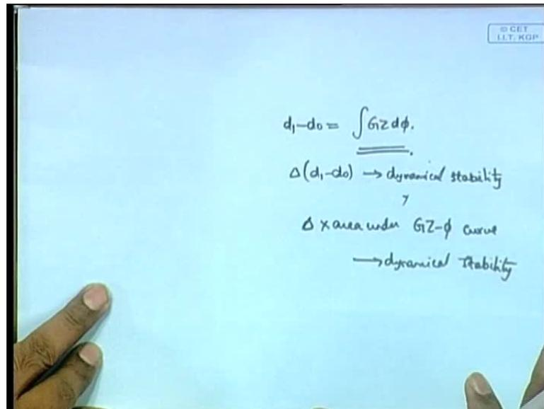
From that you get this expression that  $d_0$  minus  $d_1$  is equal to integral of  $GZ$   $d\phi$ , which is the delta into  $d_1$  minus  $d_0$ , which is known as the dynamical stability is delta times the area under the  $GZ$  curve and area under the  $GZ$  curve is the dynamical stability arm and delta into area under the  $GZ$  curve is the dynamical stability and that is known as the work done to move the ship heel - the ship that is dynamical stable.
