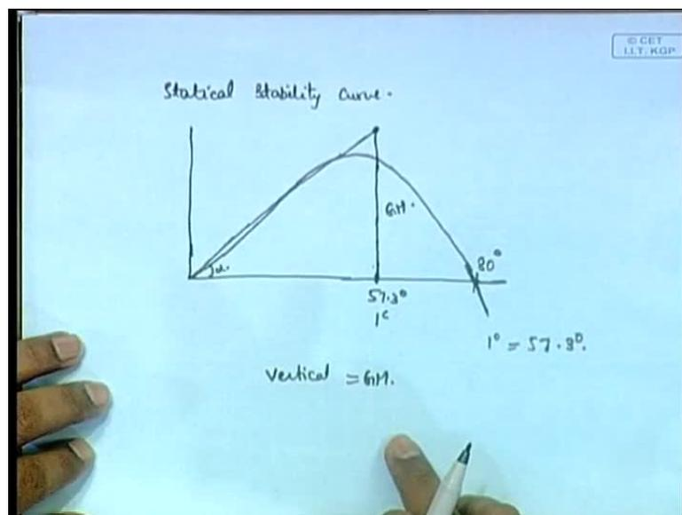
Now, I have already mentioned to you what we called as the statical stability curve or the curve statical stability. So, this goes up and comes down like this; this time it is at 80 degrees in this figure. I have already told you that at an angle of 1 radian and you should also know that 1 radian is equal to 57.3 degrees conversion from radians to degrees. At around 57 degrees that is at 57.3 degrees if you draw a line vertical and at that point somewhere here (Refer Slide Time: 06:30).
