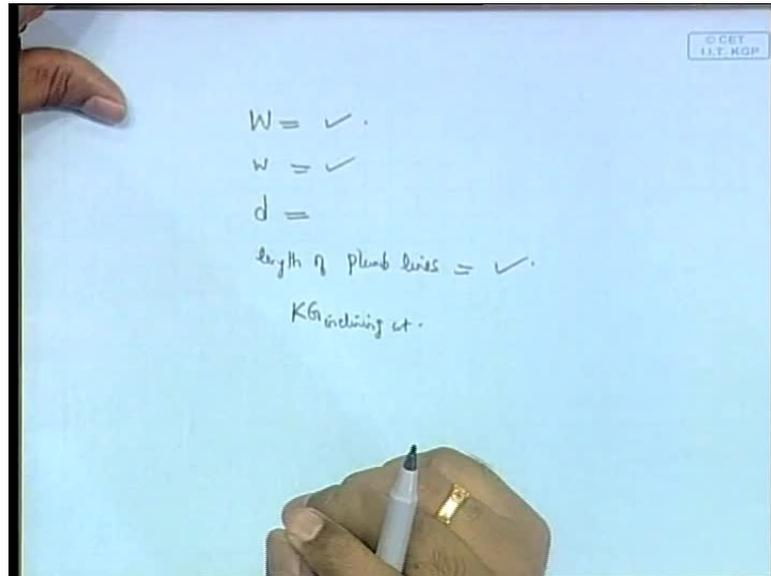
You are given the following data: you are given the displacement of the ship which is your capital  $W$ , you are given the displacement, then you are given small  $w$  the mass of the inclining weight, then you are given small  $d$  - the distance through which that small mass is translated, **then you are told just write this** the meaning of this is...length of plumb lines means the length of the pendulum - plumb line, that indicates the pendulum that is being hung there, that is given.
