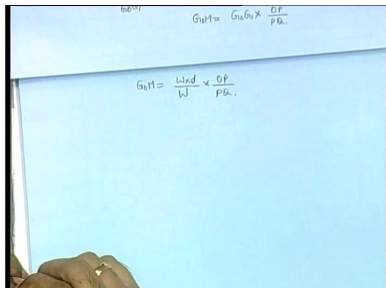
Therefore, we can say that  $G_0 M$  by  $G_0 G_1$  is equal to -  $G_0 M$  - it is equal to  $O P$  by  $P Q$  - it is just the similarity; therefore,  $G_0 M$  is equal to  $G_0 G_1$  into  $O P$  by  $P Q$ ; now,  $G_0 M$  is equal to  $w$  into  $d$  by capital  $W$  into  $O P$  by  $P Q$ , so I have just replaced  $G_0 G_1$  by that new value.
