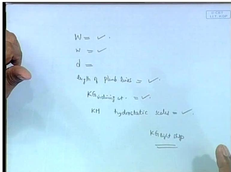
KG of that inclining weight is not the hanging weight, it does not matter how much weight you hang; inclining weight means the weight that is shifted. Inclining weight - you are given the KG of the inclining weight - and from... KM is given, otherwise you
