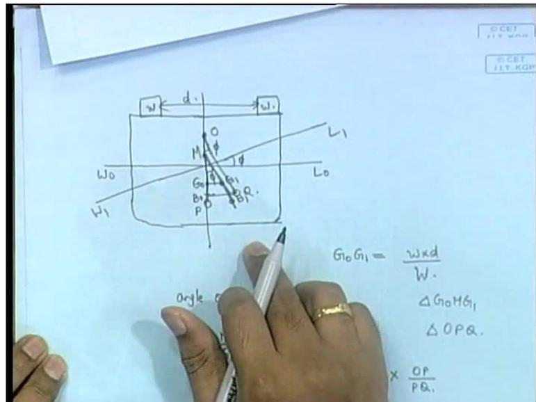
If you want to remove that weight and find just the weight of the light ship, **which is what really the KG**, which is really the GM that we should be giving as the result of inclining test; you need to subtract another KG, that is, a KG of that inclining weight alone or that shifting weight alone.
