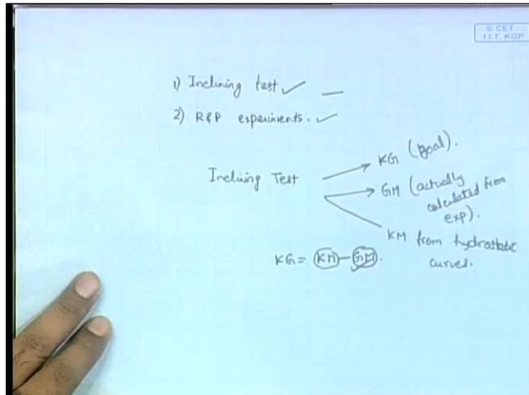
Today we will do something, which is a very important test; it is known as an inclining test or an inclining experiment. Whenever you are constructing a vessel - really constructing it in the shipyard you will see that **you need to add...** you need to do a couple of experiments; once you...so first of all you develop the hull; once the hull is developed you need to do stability calculations - you need to make sure that the stability of the ship is alright for that particular hull.
