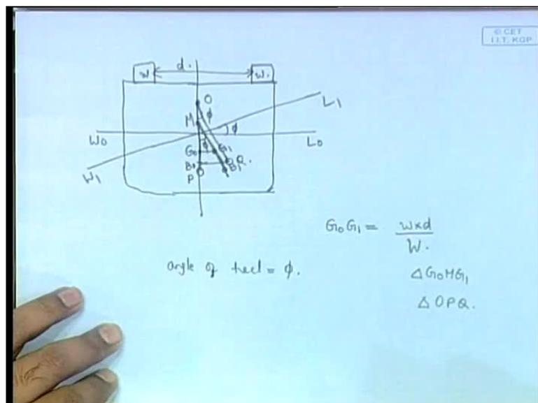
Let us explain what the test is: that is, suppose you have - this is your vessel cross section; now, what we are going to do is - this is the center line ... suppose there is a weight here of - a small weight, small w - there is a small weight there of weight small
