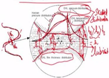
Now, comes to the elasto-hydrodynamic lubrication. If you look at these two non-conformal contacts, this is being blown up here. This is one tooth kind of things, gear tooth and this is another gear tooth. Now this is pressed against other. According to Newton's law every action has an equal and opposite reaction. If it is  $F_n$  here, it should be  $F_n$  from the other tooth also. Now, use lubricants here.
