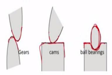
Typical non-conformal contact, for example gears. So, this is called gear tooth. So, these two teeth in the gears they essentially represent non-conformal contact. Here again cams. Again, it is a non-conformal contact. Ball bearings; This is one ball. In one of the earlier lectures, I have mentioned that one of the innovations that has happened in the field of ball bearings is
