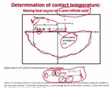
So, then the last point is that for example, how to find out that the contact temperature on a semi-infinite solid? In case of the semi-infinite solid, what will happen? Suppose if you consider that this is your contour of the solid. So, this is the contour of the solid and on which a heat source, what is a heat source? For example, Heat source can be a pin. Because pin is sliding at a distance v at a sliding at a speed v.
