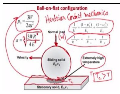
In this particular slide, what would have learned from last 1 or 2 lectures. If you look at this diagram, this is a spherical ball which is in contact with a flat surface. Both these surfaces as you can see, they are nominally flat. If you see this particular flat surface, this flat surface is also nominally flat. However, as I have mentioned couple of times during the course of last 3 lectures, that each of the surfaces whether it is sphere or flat surfaces, they have number of asperities.
