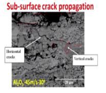
Horizontal cracks -parallel to the coating surface located at the splat boundaries and along the decomposition layer boundaries.
