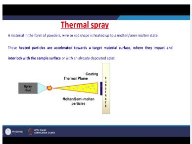
So thermal spray coating techniques are generally used for coating ceramics on a substrate. So in the thermal spray, a material is fed in the form of powders, wires, or rods and this material is heated to a molten or a semi-molten state. The heated particles are accelerated towards a target material surface where the impact and interlock with the sample surface are with already deposited splat and then the coating is formed.
