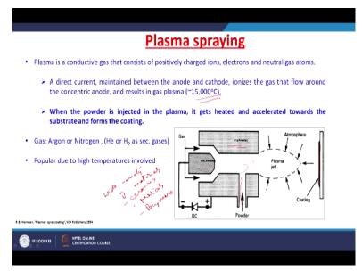
So first plasma spraying technique. The plasma is a generally a conductive gas that consist of positively charged ions, electrons and neutral gas atoms. So you have a plasma that can have a temperature of very high temperatures of around 15,000 Celsius. So how do you produce such a plasma. A direct current maintained between this anode and the cathode ionizes the gas that flow around the concentric anode and results into a plasma.
