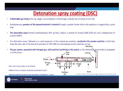
Other one is detonation spray coating. Detonation spray coating is very useful coating for coating a material on to the substrate. The material can be of ceramic or metal or a polymer. So in this detonation spray coating, a flammable gas mixture again, for example oxygen or acetylene is fed to a tubular barrel closed at one end, right. So this gas mixture is fed into this tubular barrel which is closed at one end, right.
