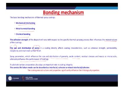
If we look at the bonding mechanism of this thermal spray coatings, generally the bonding is possible just by mechanical interlocking, the metal to metal bonding, or a chemical bonding, right. So the adhesion strength of this deposit will vary with respect to the specific thermal spraying technique that influences the microstructure of the resultant coating.
