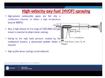
The high velocity oxy fuel spraying technique, here the high volume of combustible gases are fed into the chamber to obtain a temperature of around 3000 Celsius. At the same time, a high velocity gas stream is also required to obtain the dense coatings. So the gas stream will be
