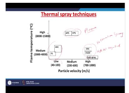
So based on the temperature, that is developed within this flame are the acceleration that is given to these particles, based on these temperature and then acceleration, there are several thermal spray techniques. Namely, the plasma spray technique, either arc plasma or vacuum plasma. There are plasma techniques and then there is an arc technique and then flame spray technique, detonation spray coating and high velocity oxy fuel.
