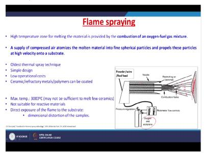
The other technique is a flame spraying technique. So high temperature zone for the melting the material is provided by combustion of an oxygen-fuel gas mixture. So generally the fuel is of acetylene gas. So oxygen and then acetylene gas mixture is given into this chamber where the powder or the wires or the rods are fed into this chamber and then combustion gives a temperature of around 3000 Celsius.
