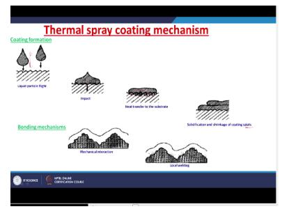
So thermal spray coating is generally done by a mechanism, coating formation mechanism. Initially as I told the particles are heated to a molten or semi-molten state. These particles impinge on the surface and then while impinging, they transfer the heat on to the substrate. In the later stages, they solidify into a coating splat. So solidification and shrinkage of the coating splats are the final result of this coating, right.
