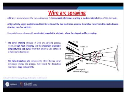
So material is fed in the form of a wire and a DC arc is struck between these consumable wire
