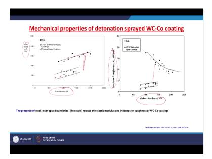
Let us see one study on the mechanical properties of detonation sprayed tungsten carbide cobalt coating, right. If you look at this one, this is the elastic modulus in gigapascal. This is Vickers hardness. Again this is the fracture toughness and Vickers hardness, right. If you look at this, data obtained from the bulk tungsten carbide cobalt, right. Whereas this data is obtained for the coatings of this tungsten carbide cobalt.
