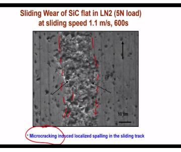
This is at the high sliding speed conditions and you can see this is your wear track and this wear track a closer look at this particular region clearly shows you that there are multiple or there is numerous microcracks so this microcracking is playing an important role in this particular case and that is the high sliding speed of 1.1 meter per second. Unlike this alumina or zirconia in silicon carbide, we have fixed the normal load of 5 Newton.
