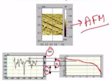
So, this is the construction of the bearing area curve. You know you can get all this 2-D profile. From the 2-D profile, you can get a bearing area curve. This is a typical AFM image, AFM stands for atomic force microscopy. That gives a very high resolution like it goes to micron scale and even lower surface roughness. And from there, you can find out that what is the valley roughness? what is the peak roughness? what is the mean roughness of the surface aspect ratio?
