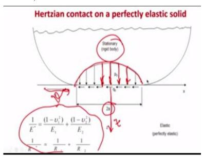
So, these are more clearly defined what I mentioned in the last slide. That how to find out an effective elastic modulus and how to find out a radius and effective radius of the surfaces. This is the case for the Hertzian contact on a perfectly elastic solid and you can see that you know how Hertzian contact that pressure is kind of varying. And you can see this is the 2a values here and this is your z and this is your traction.
