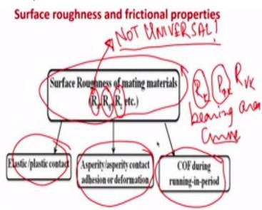
To summarize, in last half an hour or so, I have mentioned that how surface roughness of the mating materials can be effectively quantified by  $R_a$  value,  $R_q$  value,  $R_z$  values and then other
