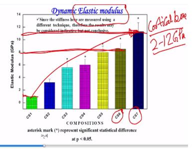
So there is also another properties which are important for tribal logical applications which I have mentioned earlier is that elastic modulus because this that is if there is a difference in the elastic modulus suddenly the different magnitude of the 809 contracts process that will be developed at the tribal logical surfaces.
