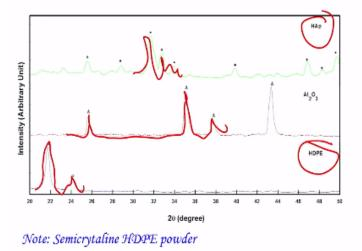
Okay so what are the different and this is the starting powder so high density polyethylene as you see this peak is little broad so therefore is a semi crystalline polymers. It is not a fully crystalline like the case for many other polymers. Now we have alumina is also crystalline peak and hydroxyapatite is a very characteristic 3 weeks which are placed around 30 degree of both values.
