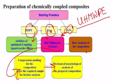
Now so far that it is one of the materials which is widely used in the acetabular socket application is ultra-high molecular weight polyethylene Now ultra-molecular polyethylene has a higher molecular weight so higher the molecular weight the mode is the viscosity and mode is the viscosity means more difficult would be these polymaths to process Okay so if you want to add some new materials or if you want to add some new phases like ceramic phase
