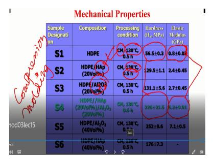
But what is more important for you to see here and realize that high density polyethylene alone has a hardness of <100 megapascals when you go to high density polyethylene 20% have 20% alumina the hardness goes almost like 4 times higher than their compared to baseline elasticity. In terms of elastic less which is more important for biomedical applications as well as for tribal logical applications it shows an increase from 0.8 giga pascal to 6.2 giga pascal.
