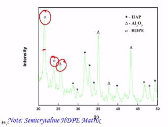
So when you add these two phases like 20% hydroxyapatite and 20% the alumina you get a very clear semi crystalline peak but this peak which is little bit decreased. Now in the compression molded samples and you have a hydroxyapatite and you have alumina phase as well.
