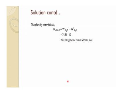
Similar way we can then calculate if we subtract the one which is coming with the feed; the actual amount which should be added is about 64.51; 51 k kilogram per metric ton of wet mix And in the previous one it was 65; so, about 1 kg difference which is coming out.
