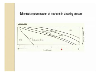
And if we talk about little bit about the heat transfers here. So, that is the thing which we discussed the condensation is occurring. After that in this zone because the moisture which has evaporated re condensing in the lower temperature zone, you have a sintering zone about 1200 degree c then you have a heat front cooling zone and the top one really from the atmospheric air gets cooled down below this 40 degree.
