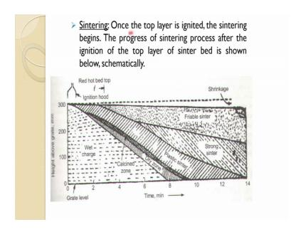
So, once the top layer is ignited the sintering begins the progress of sintering process after the ignition of the top layer of sinter bed is shown below schematically. So, there is a so, when the process I think probably it can be understand much better way from this figure how these zones.
