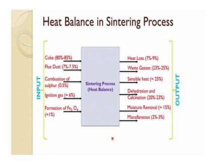
And for the heat balance we have this. So, in the heat balance 80 to 85 percent heat comes from the coke and a flue dust constitute that about 7 percent combustion of sulphur about 0.5, ignition of gases also through the burner its about 6 percent and a formation of F e 3 O 4. So, from hematite to magnetite it is a exothermic process essentially. So, about 1 percent comes from that and total heat loss.
