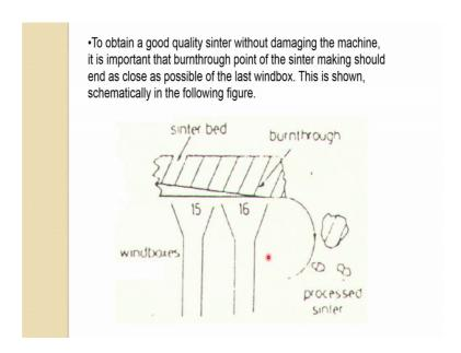
So, the main now one important thing is you look at this; we are having at the flame front. If flame front is going to continue like this then it is going to really under temperature 13; 1400 degree Celsius and that is going to damage the strand and the hearth.
