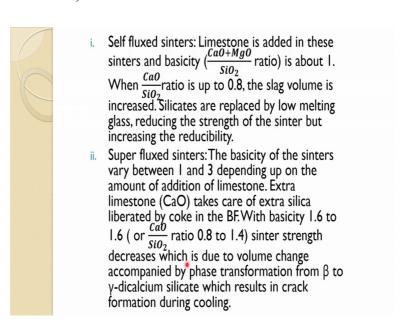
So, basic sinter this flux sinter or further classified into again various basicity based on their basicity ratio. So, self flux sinter where the ratio of the basis this basic and acidic compound is about 1, we say basicity 1. So, so and in terms of Ca SiO 2 if it is about 0.8; so, so this actually called the self flux sinter.
