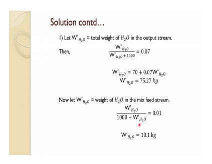
So, if the total weight of water in the output stream. So, this we can is a W naught H 2 O; if that is the total weight. So, normal mass balance of the water will give W naught divided by this and weight of the water should be 0.7. So, if we solve this; so, essentially what we get the amount. So, 1000 is coming and because we are doing an metric ton basis.
