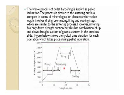
Otherwise most and you can see from this figure how the different phenomena are occurring; how much time it takes. So, drying about 10 minutes preheating another 5 minutes and mostly then the firing about 10 minutes takes and then the cooling. So, these are the sort of steps which similar to the sintering one. So, only the problem you have a combination of down and up draft here.
