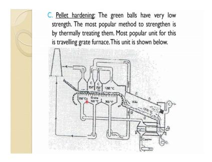
So, it goes to pellet hardening process in the previous one it is first going to the sintering one, in this one it is a pellet hardening. So, individual pellet usually they keep their shape in this case. So, it is not the fusion stage; so, temperature is little lower in this case. So, as you will see the this figure shows the in duration machine.
