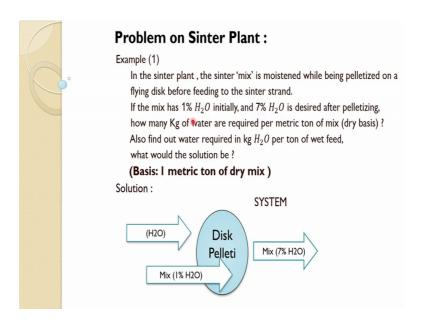
Now, there is one problem on this sinter plant which is given here. So, the example one; so, this says in the sinter plant the sinter mix is a moistened while being pelletized on a flying disc before feeding to the sinter strand. If the mix has 1 percent of water initially
