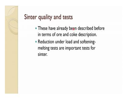
So, these we already discussed during the iron ore and coke description; so, not going to repeat really, but some important one is that reduction under load and softening melting test are important one in the in the sinter which are routinely carried out to check its quality.
