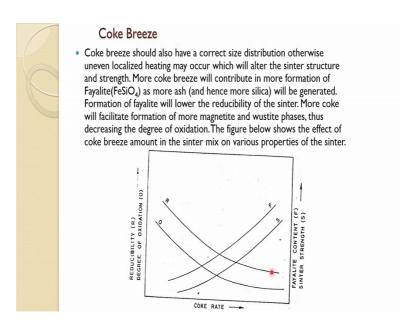
So, 8 percent for the pellet it is a good one for coke breeze; so, this should have a correct size distribution otherwise uneven localized heating may occur. Because these all are fines and when you are looking at these particles 2 millimeter and 3 millimeter particle; so, the way heat would be released, it is sort of a localized in the within the pellet.
