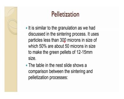
Now, we will come to the palletization as I said this is another name of the granulation we can say. So, it is similar to the granulation as we had discussed in the sintering process; only difference it uses a particle less than 300 micron size and in which 50
