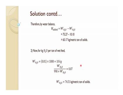
So, that gives you about 65.17 kg per metric ton of solid. Now in terms of wet feed we are already we have put 0.1 I am saying 1 metric ton. So, essentially 10 kg of water we have supplied in the feed is carrying over that much. So, again if we do the mass balance and W naught the way we have defined here the weight of the water in the final feed; the simple mass balance will gives you now this 10 kg has to subtracted from 1000. So, essentially dry this over is 990.
