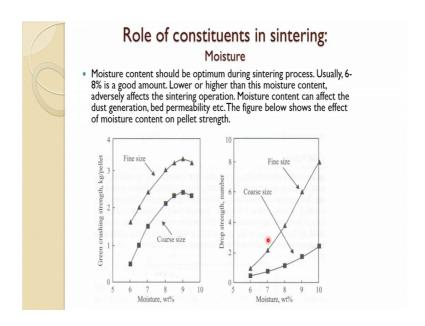
Now, we will talk a bit about the constituent role of constituents in sintering. So, as you know we have moisture during the granulation process. So, moisture content should be optimum during sintering process usually 6 to 8 percent usually in sintering process it is about 6 percent, but in palletization its a little higher it goes around 8 percent or so.
