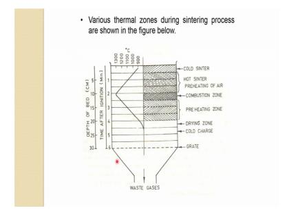
So, in the starting you have a green pellet once this under the ignition hood this sintering is start from the top it comes it comes out that. So, this is all ready now top one is a sintered one, but because the wind works are located at the bottom; so, it is sucking the air the fresh air atmospheric one from the top. So, due to the forced convection we will talk a little bit about the heat transfer later.
