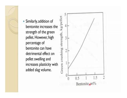
Ah Now bentonite when we said as you increase the bentonite, you can see the green crushing strength is increased which is actually a good, but you cannot use a very high bentonite because it gives a detrimental effect on pellets swelling and increase the plasticity with added slag. So, up to some extent it is fine; sometime even molasses is also used in place of bentonite.
