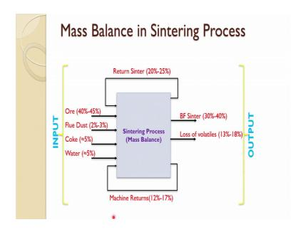
And typical mass and heat valance on that sintering process is given in this one. So, the mass valance about 40 to 45 percent all goes in 2 to 3 percent fine dust about 5 percent coke and about 5, 6 percent water it goes and the return sinter return the return fines which also comes its about 20 to 22 percent
