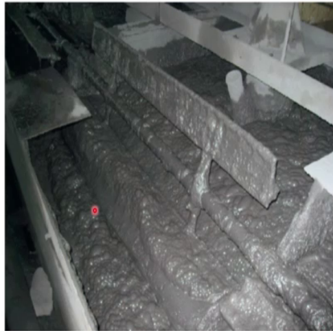
Flotation cell for iron ore beneficiation
