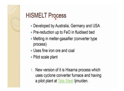
Beside these two there is no other process has the commercial plant. Now Hismelt is a promising one this is started by a C R A Australia long time ago. And then Germany and USA also joined later on in the development of it. So, this is again also based on the fines iron ore and coal.
