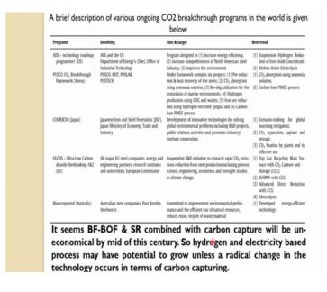
So, this lots of efforts worldwide that go going on to reduce the CO 2 and the steel plants and there are various technologies which are being developed. So, this figure can you saw the brief description of various ongoing CO 2 breakthrough program in the world. So, there is one American AISI technology roadmap. So, in this one mostly that increase the energy efficiency competitiveness in North American steel industry improves the environment.
