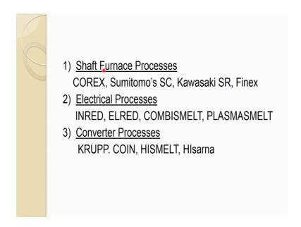
So, shaft, shaft furnace process COREX Sumitomo's Kawasaki Electric Arc, these are smelting reduction processes.
