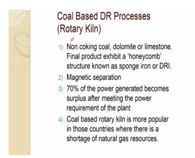
So, the these are sort of the condition in that rotary kiln and non coking coal dolomite or limestone and final product exhibit a honeycomb structure. So, with that is why you usually call it as a sponge iron or DRI magnetic separation is used to separate it with the waste and 70 percent of the power generated becomes surplus after meeting the power requirement.
