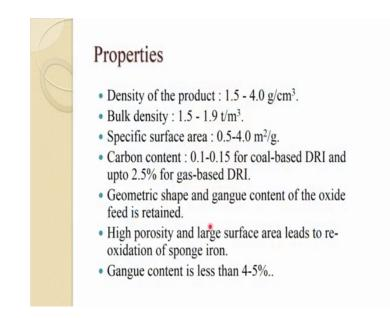
Usually the density of the product then this between 1.5 and 4 gram per centimeter cube or 1500 to 4000 kg per meter cube bulk density 1.5 to 1.910 again the tonne per meter cube specific surface area is about 0.5 to 4 meter square per gram carbon contains usually it is range between 0.1 and 0.15 for coal based DRI and up to 2.5 for gas based DRI. So, essentially as you can see till it is quite low the percentage of carbon into it. So, the melting point in that way becomes bit quite high.
