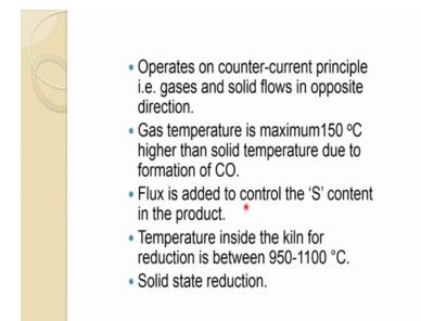
So, it is operates on counter current principle because the solid is coming from the direction gates are passing from that. So, it is a counter current principle gasses and solids flows in opposite direction gas temperature is maximum 150 degree Celsius higher than the solid temperature due to the formation of co.
