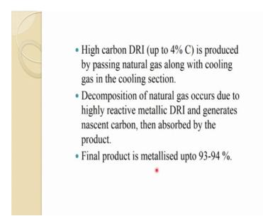
Melting point high carbon DRI up to four percent is produced by passing natural gas along with cooling is in the cooling gas section. So, you see the here natural gas along with the cooling you can get a high percentage of carbon which it probably the product reaction which we show to carbon deposits in the reaction may occur in and can increase it.
