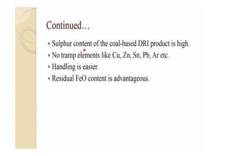
Sulphur contained especially in the coal way DRI product is quite high, because there is no slag can take it. So, most of the sulphur content is retained in to that. So, it is usually quite high no tramp elements like copper, copper, zinc, tin, lead, arsenic, and etcetera. Handling is easier as a solid product. The residual FeO content is advantageous. So, some of the iron which is not reduce or the reoxidation is appear is formed.
