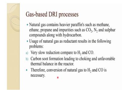
Imported hydrogen is faster than the carbon monoxide. So, natural gas contains heavier paraffin's such as methane, ethane, propane and impurities like carbon, nitrogen, sulphur, compound along with hydrocarbon.
