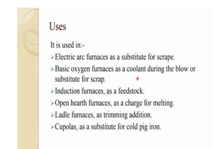
Is usually electric arc furnace as a substitute for a scrap no? So, that for the scrap and the electric arc furnace when the scrape is not there it can be substitute for that for steelmaking. Similarly in the basic oxygen furnaces it is used as a coolant during the blow or substitute for scrap.
