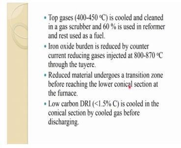
So, top gas temperature is between 400 and 450 degree Celsius this cooled and cleaned in a gas is scrubber and 60 percent is used in reformer and rest is used as fuel as I said some coals are again back with that and some coals as a fuel.
