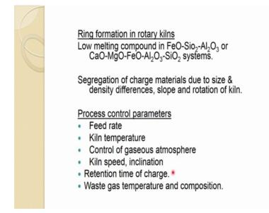
The problem which is associated with this very often is a ring formation that ring formation into to the low melting compound of this iron silicate, aluminate, SiO 2 big oxygen ore, calcium, magnesium, iron oxide or not SiO 2 system that forms a low melting compound and which deposited around near on the wall of this and that forms a ring and that is why taking a rotaring formation which it is a ring information and that have major problem in this.
