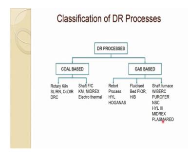
Now, the classification of direct reduction processes we talked a lot about the gas natural gas as a reducing agent and then coal as reducing essence so; obviously, there are two classification of direct reduce process 11 is the coal based and another is gas based and coal based processes like Rotary Kiln SLRN there are many processes which are based on this then shaft like processes KM MIDREX Electro thermal I had. So, rotary can type with this shaft type of this.
