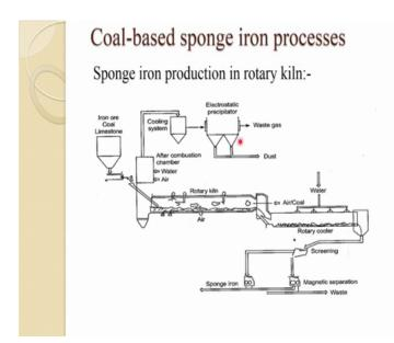
Rotary kiln which we said even slr and it is under same principle. So, sponge iron production in rotary kiln so, what essentially in this it is done that iron ore coal and limestone. So, like it sort of a composite they are mixed together and feed it sort of a composite pellet, spoon and they are put through to choose to the rotary kiln and they are case which is supplied through that and some time with the burners through which the fuel is supplied and mostly from this exit side.
