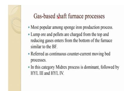
Based processes so, most popular among sponge iron production processes. This gas based one lump ore and pellets are charged from the top and reducing gases enters from the bottom of the furnace similar to the blast furnace. Referred as continuous countercurrent moving bed processes.
