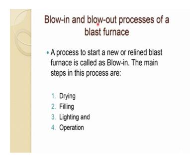
So, there are two important operations in the blast furnace, one is blowing and another is blow out processes of a blast furnace. So, if process to start a new or relined blast furnace is called as blow in. So, whether it can be a new furnace or it could be even a relined one. So, the main steps in this process are.
