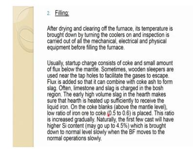
So, as we mentioned in the previous in this slide that any ratio of iron ore to coke is 0.5 to 0.6 and slowly it increases 0.05 or 03 sort of ratio slowly and another way of doing it to analyze the CO-CO 2 ratio and based on that as you can slowly increase the iron ore content into the charge.
