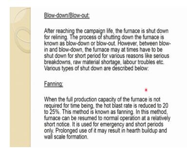
So, like blow in we also have the operation like blow down or blow out. So, blow down and blow out is after reaching the campaign life, the furnace is shut down for relining.
