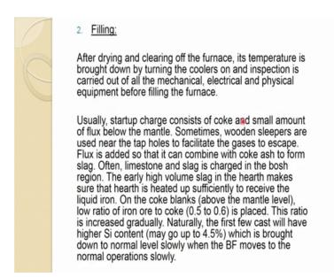
The second step consists of filling. So, after drying and clearing off the furnace clearing off the furnace if you have used the second method or some others. So, you have to remove whatever is left over there. And clearing off the furnace its temperature is
