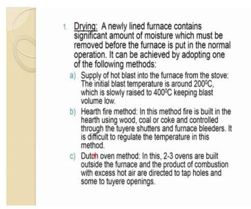
So, the first step is drying. So, a newly lined furnace contains significant amount of moisture which must be removed before the furnace is put in the normal operation. So, this is a very critical step and very important and one has to make sure all moisture must be driven away.
