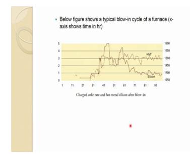
So, some of this figure shows a typical blow in cycle of a furnace. So, x axis this is showing hours this. So, the silicon content in percentage and that is the hot metal temperature.
