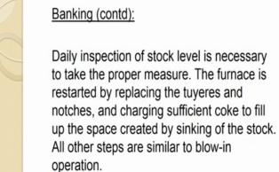
So, daily inspection of stock level is necessary to take the proper measure. The furnace is restarted by replacing the tuyere and notches and charging sufficient coke to fill up the space created by sinking of this stock.
