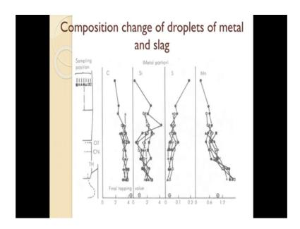
This gives an again idea again from a dissected blast furnace, the change in the composition of metal droplet of metal and slag. So, these are sort of a sampling position from where they picked up, the metal and slag droplets and as you can see this is actually the sort of tuyere region. So, temperature is high in this region.
