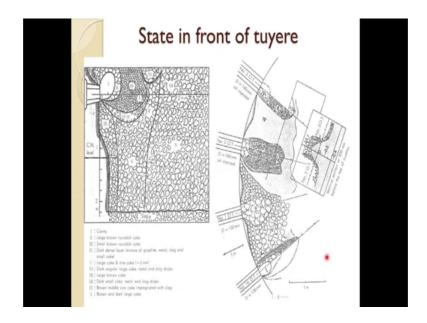
Now, this again about the dissection of that blast furnace and when they look at the raceway region, because that is a very important reason on which, the whole reduction permeability aerodynamics of the blast furnace defense.
