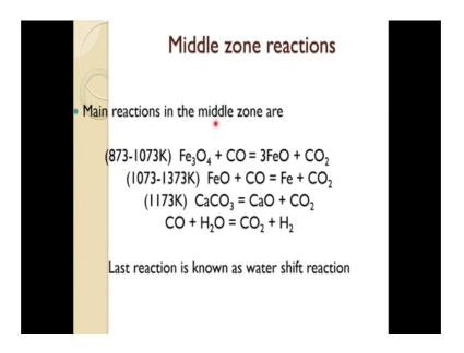
Through the case and the middle zone reaction, the main reaction again some magnetite to wustite, it reduces and from wustite to iron. So, most of the iron get reduced in this region, but not all may be up to 70 percent or. So, and calcium carbonate decomposes in this region and this C O 2 react with the carbon, and from C O again and even they whatever some moisture is there, that also react with the C O and keep C O 2 and hydrogen, and as you know hydrogen is much better reductant than C O.
