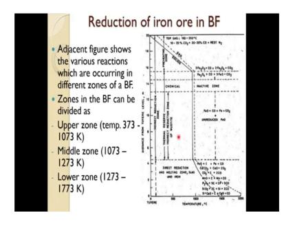
The direction of iron ores and blast furnace so, this figure shows the various reaction which are occurring the blast furnace, as we which is you know there various region the throat region, as we said throat throat region, stack region, belly region, bosh and hearth.
