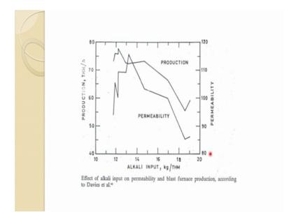
And due to this alkali input as we said that because the permeability increased. As you can see as the alkali input increases in kg per tonne of hot metal, it will adversely affect the permeability of the burden and similar then the production will go down. So, productivity also decreases. This is quite clear from that. So, alkali percentage should be kept minimum as much as possible in the raw material. So, like a beneficiation other thing can take care of it.
