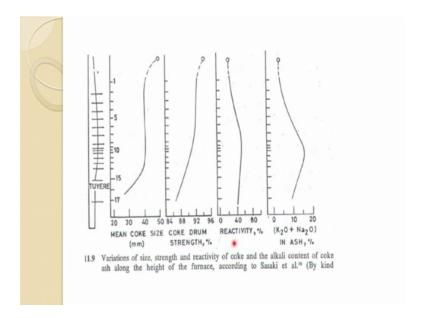
So, this is a tuyere level. If you look at coke size, so you will see that the tuyere level, the cock size is about 25 or 30 millimeter. So, you are feeding about 50 millimeter soil and they starting. And by the time it comes to the tuyere region, it reduces almost 50 percent. And even if it reduces 50 percent, one has to make sure this coke because this is the
