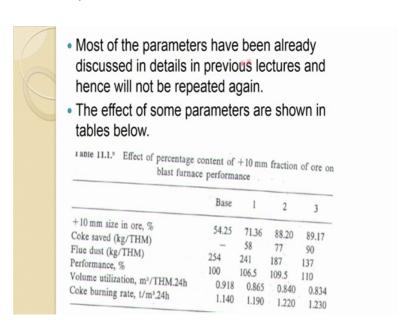
So, most of the parameter we have discussed in previous lecture so not repeated again. The effects of some parameters are shown in this table. So, effect of percentage contents of plus 10 millimeter fraction of ore in the blast furnace. So, Base condition is this. So, plus 10 millimeter not it is 54 percent. If you increase that one to 71 percent, so savings you can see. How much? 58. This these are actual plan data.
