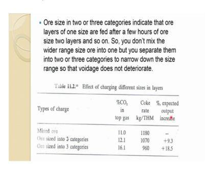
So, ore size also, now we said only 1 plus 10 millimeter, now see the effect of different ore size. So, ore size in two or three categories indicate that ore layers of one size are fed after a few hours of ore size two layers and so on. So, you do not mix the wider range size ore into one but you separate them into two or three categories to narrow down the size range so that voidage, voidage does not deteriorate.
