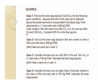
So now, we will come to the example which we were talking about. So, let us have a general thing first find out the bosh slag basicity that is CaO to SiO2 ratio for the following given condition. So, assume that 30 percent of the coke ash is released above the tuyere level and is incorporated in the Bosh slag. Final slag basicity is 1.1, so that is given.
