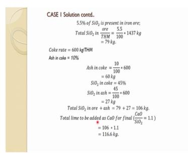
So, 5.5 percent of SiO2 is present in the iron ore. So, total SiO2 would be is multiplied this convert it into small friction or friction. That multiplied with iron ore per tonne basis which is needed. So, you get 79 kg of SiO2 which is present in 1437 kg of iron ore. Now, coke rate is given 600 kg per tonne of hot metal and ash contained in it is 10 percent.
