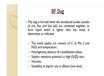
So now we would focus mode on the blast furnace slag. So, what we have discussed till now a general properties of the slag and the liquid iron. So, in blast furnace the slag is formed when the unreduced oxides like oxides of ore flux and fuel ash are combined together to form liquid which is lighter than the hot metal. So, it determines or indicates the metal quality content of carbon silicon manganese sulphur and FeO and temperature.
