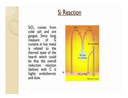
So, we will be talking a little bit more about it. So, because historically if you see we will see here, SiO 2 comes from coke ash and ore gangue and since long measure of silicon content in hot metal is related to the thermal state of the hearth, which could be that the overall reduction reaction with carbon is highly endothermic and slow.
