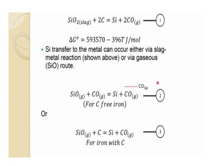
So, this normal that reaction in the hearth reason, we set with the slag and the carbon keep this is you can say even dissolved carbon or normal with metal or normal carbon that gives you the silicon which its dissolve into iron and 2 CO so; obviously, the reaction is quite endothermic this. So, this endothermic nature of the reaction you need that temperature in this.
