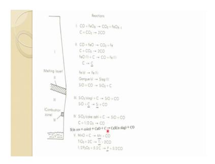
So, if you look at the blast furnace in the stake region you have a various form of iron oxides which get reduced into the lower one and whatever CO 2 formed it goes into CO and this a cohesive zone, because once the solid comes up to here mostly you get the boost tight in this region. So, CO reacted with tight.
