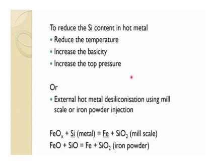
So, in summary I would say also to reduce the silicon content in hot metal, reduce the temperature increase the basicity increase the top pressure or if you needed really very lost silicon content it is not possible through that, then external hot metal desiliconisation is necessary, which can be done using milli scale or iron powder injection in either in a torpedo car or other out outside process.
