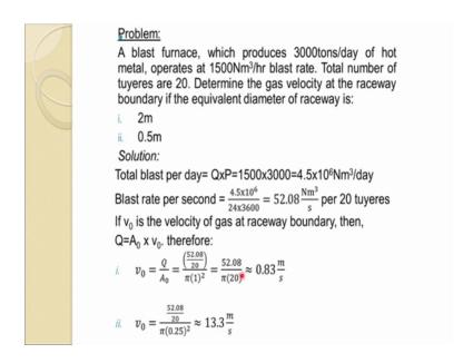
So, there is one problem. So, a blast furnace which produces 3000 tons per day of hot metal, operates at 1500 normal meter cube per hour blast rate.
